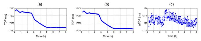
**Fig. 5** Absolute TOF between acoustic path lengths traversing (a) an empty cassette and formalin and (b) only the formalin. (c) Reference-compensated TOF calculated as the difference between (a) and (b). Stable reference-compensated TOF demonstrates robust environmental mitigation ( $\sigma = 247$  ps).
