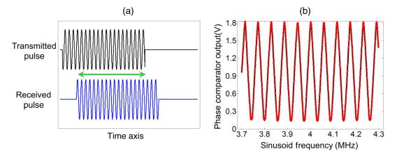
**Fig. 3** (a) Qualitative depiction of transmitted and detected acoustic pulses. (b) Output voltage of phase comparator versus frequency of the transmitted sinusoid representing the phase relationship between transmitted and received signals. Values generated during region of overlap (green arrow). Red stars are recorded data points (v = 3.7 to 4.3 MHz,  $\Delta v = 600$  Hz). 0 V =  $\pm \pi$  rad, 1.8 V = 0 rad.
