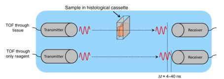
Fig. 1 Schematic representation of the acoustic TOF diffusion monitoring system. Transit times of acoustic pulses traversing the formalin and tissue (top row) and a reference acquisition through only the formalin (bottom row) were calculated. Reference channel subtraction eliminated environmentally induced noise and isolated the TOF contribution from the tissue.
