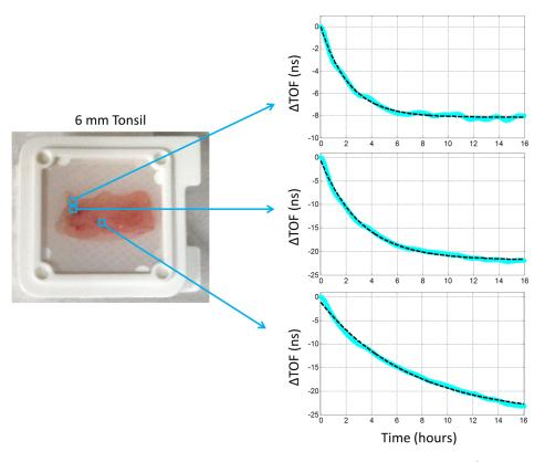
**Fig. 6** Measured  $\Delta$ TOF from regions in a 6-mm human tonsil completely diffused (top,  $R_{adj}^2 = 0.994$ , SE = 145 ps), mostly diffused (middle,  $R_{adj}^2 = 0.996$ , SE = 320 ps), and partially diffused (bottom,  $R_{adj}^2 = 0.996$ , SE = 406 ps) after 16 h in formalin. All  $\Delta$ TOF offsets were subtracted off.
