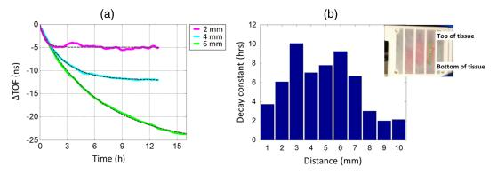
**Fig. 8** (a)  $\Delta$ TOF from tonsil samples 2 mm ( $R_{adj}^2 = 0.8$ , SE = 350 ps), 4 mm ( $R_{adj}^2 = 0.999$ , SE = 90 ps), and 6 mm ( $R_{adj}^2 = 0.998$ , SE = 230 ps) thick in 10% formalin. All  $\Delta$ TOF offsets were subtracted off. (b) Decay constants from 6-mm tonsil, obtained sequentially from top to bottom. Decay constants range from 2 to 10 h ( $\sigma$  = 2.9 h).
