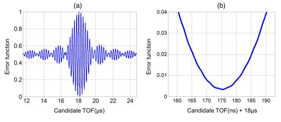
**Fig. 4** (a) Normalized error function versus candidate TOF. Function resembles an optical interferogram. (b) Error function near global minimum, which corresponds to the true absolute TOF.
