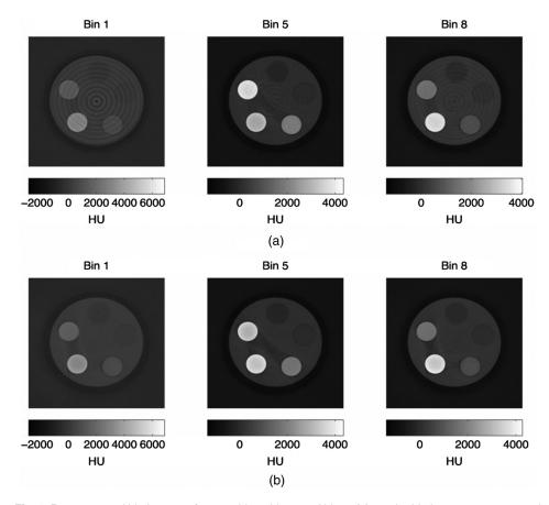
**Fig. 8** Reconstructed bin images of energy bin 1, bin 5, and bin 8. (a) are the bin images reconstructed from the raw projection data that are normalized by flat fielding using an air scan. (b) are the bin images reconstructed from the projection data that are processed with the inhomogeneity compensation method. All images are normalized to HU measured in the water insert.
