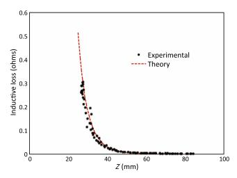
**Fig. 11** Inductive loss measured along a vertical line above the center of a  $40 \times 40 \times 6$  mm conductive square  $\sim 4.35$  S/m. Theoretical maintains perfect centering over the conductive square while the hand scan does not, contributing some variability.
