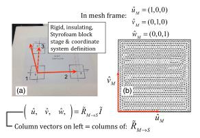
**Fig. 5** Mesh CS: (a) three position measurements define the mesh CS on the Styrofoam stage and (b) construction of unit vectors on Styrofoam stage.
