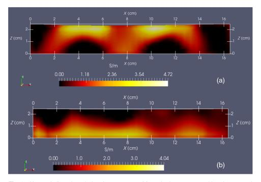
**Fig. 12** Y-normal slices through the phantom center: (a) conductive squares positioned at top and (b) conductive squares positioned at bottom.
