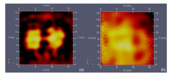
**Fig. 14** Z-normal slices: (a) slice obtained at  $Z = 20 \, \text{mm}$  (or 4-mm depth) with conductive squares at top and (b) slice taken at  $Z = 4 \, \text{mm}$  (or 20-mm depth) with conductive squares at bottom. Refer to Figs. 12 or 13 for corresponding scales.
