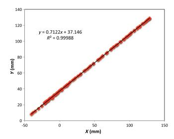
**Fig. 10** Result of a scan that tracks a nearly diagonal path along the upper surface of the Styrofoam stage, maintaining contact between coil and Styrofoam stage.
