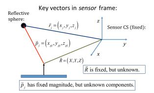
**Fig. 3** As shown, vector  $\vec{R}$  is fixed, but unknown; vector  $\vec{p}_j$  is variable but has fixed length; vector  $\vec{r}_j$  is acquired from the sensor via RS-232 and locates the reference sphere. All vectors are in the frame of the sensor CS; CS, coordinate system.
