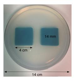
**Fig. 9** Phantom consisting of buried Play-Doh squares, immersed in agarose gel. Square inclusions are 4 cm on edge and buried to a depth of ~14 mm beneath agarose.
