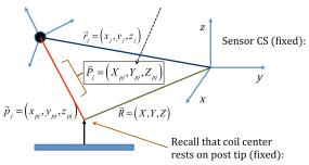
**Fig. 4** Illustration of relevant vectors—those in the frame of the fixed IR sensor and the single vector  $\vec{P}_i$  in the frame of the optical body.
