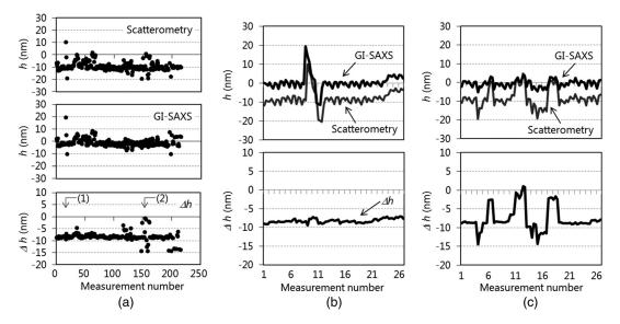
Fig. 7 Long-term evaluation results for VMS: (a) long-term evaluation results for three tools, (b) detail data at region 1, and (c) detail data at region 2.
