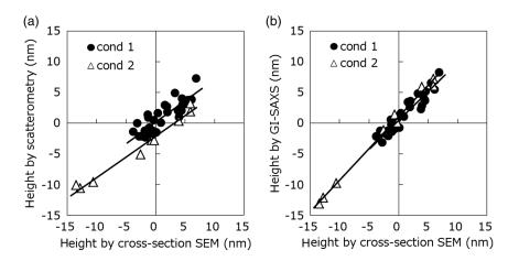
Fig. 6 Measurement robustness of scatterometry and GI-SAXS: (a) scatterometry result and (b) GI-SAXS result.
