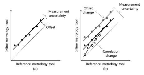
Fig. 1 Measurement uncertainty (MU) for ideal and actual pattern shapes: (a) ideal pattern shape without process variation and (b) actual pattern shape with process variation.
