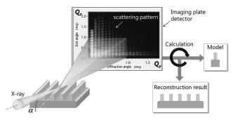
Fig. 4 Schematic diagram of GI-SAXS.
