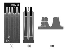
Fig. 5 Structural models for scatterometry and GI-SAXS: (a) crosssectional SEM image, (b) scatterometry model, and (c) GI-SAXS model.
