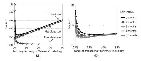
Fig. 9 Cost analysis results for false alarm case: (a) total cost for 6-month shift interval and (b) shift interval dependence on total cost.
