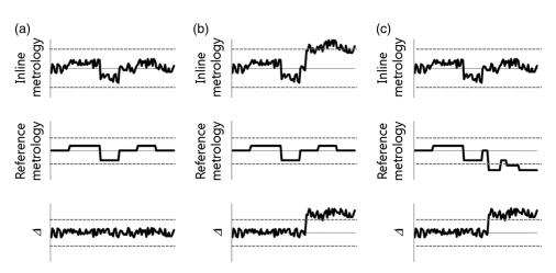
Fig. 3 Case study examples of VMS applications: (a) stable case, (b) false alarm case, and (c) nondetectable case.
