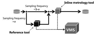
Fig. 2 Conceptual diagram of VMS.
