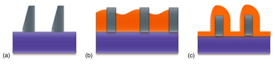
Fig. 1 Process-embedded asymmetry. (a) Asymmetric sidewall angle caused by etch. (b) Asymmetric trench caused by chemical-mechanical polish (CMP). (c) Asymmetric layer deposition caused by chemical vapor deposition (CVD) deposition.
