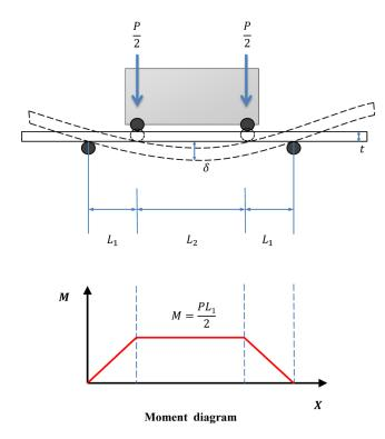
Fig. 2 Schematic diagram of the four-point bending moment.
