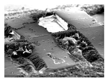
**Fig. 5** The glue flow in the structure of an SLPFG without a surface bonding layer after the surface bonding process.
