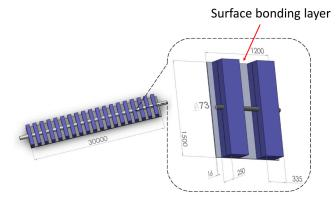
Fig. 1 Schematic diagram indicating the sizes of the different parts of the optical fiber strain sensor based on sandwiched long-period fiber gratings (OFSS-SLPFG).
