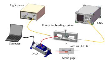
Fig. 4 Experimental setup of the four-point bending test.
