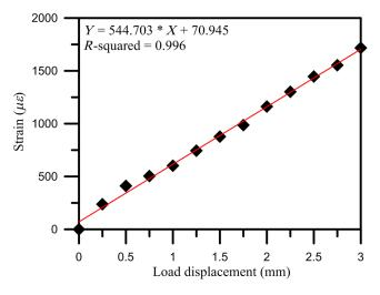
Fig. 7 The relationship of screw displacement and strain.
