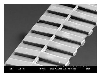
**Fig. 6** The surface bonding layer of the OFSS-SLPFG prevents the glue from flowing into the structure of the sensor.
