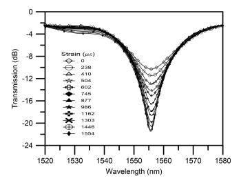
Fig. 8 The transmission spectra of the OFSS-SLPFG with various applied strains.
