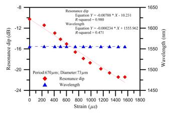
Fig. 9 Transmission and resonance wavelength versus applied strain.
