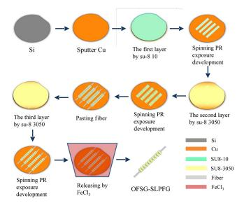
Fig. 3 The OFSS-SLPFG fabrication process.
