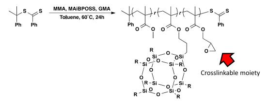
Fig. 6 Scheme of PMMA-r-PMAIBPOSS-r-PGMA preparation.
