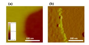
Fig. 12 BCP behavior on bare Si wafer. (a) Height image of annealed BCP film and (b) amplitude image of etched film.
