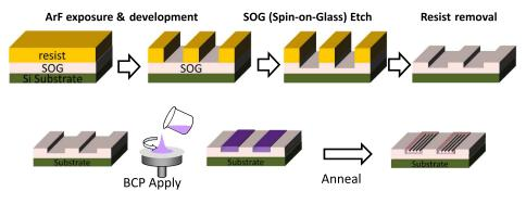
Fig. 3 Guide preparation and applying BCP process image.
