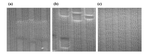
Fig. 5 SEM images of defects observed in one test chip. (a) BCP overflow, (b) nonfilled, and (c) line-edge roughness.
