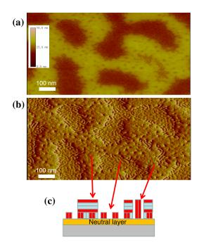
Fig. 10 Atomic force microscope images of etched BCP film surface. (a) Height image, (b) amplitude image, and (c) schematic image of cross section.
