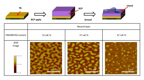
Fig. 8 Atomic force microscope (AFM) images of annealed BCP film surfaces and schematic image of BCP on PMMA-*r*-PMAIBPOSS-*r*-PGMA films.
