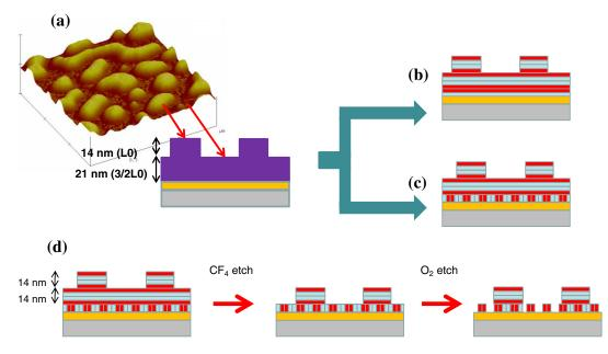
**Fig. 9** Expected images of phase-separation structure of BCP on NL and schematic image of dry development process. (a) AFM image and schematic image, (b) horizontal orientation, (c) partially perpendicular orientation, and (d) examined etch process.
