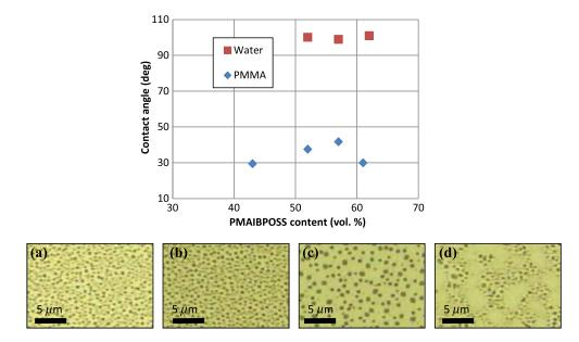
Fig. 7 Water and PMMA contact angles on PMMA-*r*-PMAIBPOSS-*r*-PGMA film surface and photographs of PMMA dots on the random copolymers. (a) PMAIBPOSS content 43%, (b) 52%, (c) 57%, and (d) 61%.
