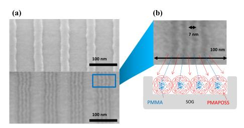
**Fig. 4** Scanning electron microscope (SEM) images of graphoepitaxy guide pattern and PMMA54-b-PMAEtPOSS10 in trench guide. (a) Top-down SEM images of guide pattern and BCP in trench and (b) magnified SEM image and schematic image of cross section.
