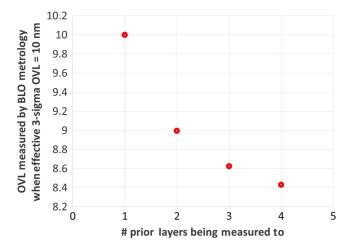
Fig. 9 The effects of Eq. (36) demonstrating that measured overlay error appears smaller as more prior patterns are used. The real overlay error stays the same at 10 nm.
