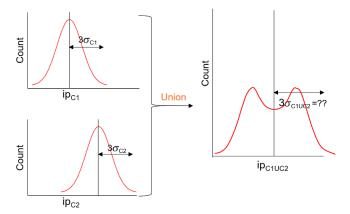
Fig. 6 When two distributions C1 and C2 combine, if they have the different means, counts, or standard deviations, the standard deviation of the combined distribution can be estimated utilizing Eq. (16).
