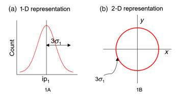
**Fig. 1** (a) A one-dimensional representation of the image placement error in one orientation and (b) a two-dimensional representation of the image placement errors in both X and Y.  $\overrightarrow{ip_1}$  is the image placement error and  $3\sigma_1$  is three times the standard deviation of the image placement error.
