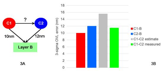
**Fig. 3** (a) The case where a overlaying pattern C is exposed with two masks each minimizing overlay error to prior pattern B. C1 to C2 overlay error is "second order" but a RSS of the standard deviations of C1 to B and C2 to B overestimates the overlay error between C1 and C2 as shown in (b).
