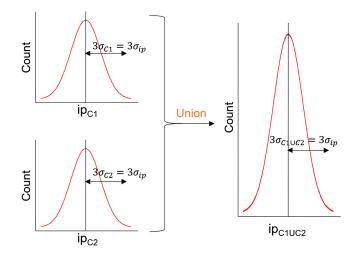
**Fig. 5** When two distributions C1 and C2 combine, if they have the same means and standard deviations, the new distribution will have the same standard deviation.
