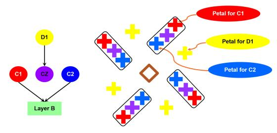
**Fig. 8** Measuring overlay error back to prior patterns can be accomplished by measuring back to all prior patterns utilizing overlay metrology structures such as Blossom. The purple "CZ" target is a virtual target that is placed in this figure to assist in understanding why when measuring back to both C1 and C2 simultaneously with a multipattern target the true overlay error can be undermeasured.
