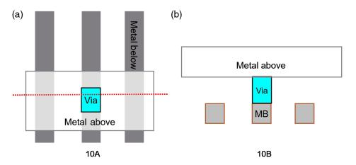
**Fig. 10** (a) and (b) A via last dual damascene integration layout where the via should be aligned to the MB even though the metal above was the layer patterned immediately before the via. (a) The design layout and (b) a cross-sectional illustration where the cross-section location is noted by the dotted red line in (a). Note that even though the via was the last patterned layer it still connects (is between) the two metal layers.
