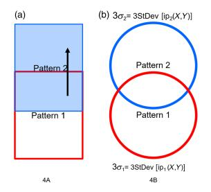
**Fig. 4** (a) The exposure fields of two patterns 1 and 2 that have a translation error in the *Y* orientation and (b) while there is the average translation error shown in (a) there is also overlay error variation within each field due to the image placement variation of each pattern.
