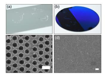
**Fig. 3** (a) Representative optical image of a peeled nanocup transparent film and (b) the metallized wafer after peel-off. (c) High-magnification (scale bar: 200 nm) and (d) low-magnification (scale bar: 1000 nm) scanning electron micrographs of the metallized wafer after peel-off.
