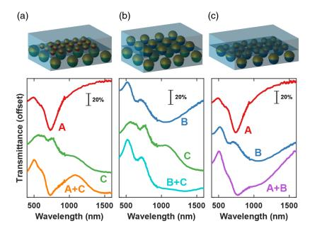
**Fig. 5** Transmittance spectra of individual films (A: red, B: blue, and C: green) and two layer stacked films for (a) 90-nm and 450-nm nanocups (A + C, orange), (b) 210-nm and 450-nm nanocups (B + C, cyan), and (c) 90-nm and 210-nm nanocups (A + B, purple).
