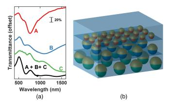
**Fig. 6** (a) Transmittance spectra of three individual gold nanocup films transferred (A: red, B: blue, and C: green spectra) and stacked in three layers (A + B + C). The plasmon resonance of interest for each individual film is indicated by an arrow. The resulting spectra after stacking are shown in black. (b) Cartoon schematic of the three layer stacked film, where complete encapsulation of the nanostructures by the pressure-sensitive adhesive film is assumed.
