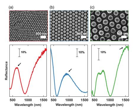
**Fig. 2** Scanning electron micrographs and reflectance spectra of periodic arrays of gold nanocups bound to a gold-coated silicon substrate (before peel-off) with an average diameter and spacing of (a) 90-nm diameter/170-nm spacing, (b) 210-nm diameter/280-nm spacing, and (c) 450-nm diameter/580-nm spacing. An arrow indicates the plasmon mode of interest. Scale bar: 500 nm.
