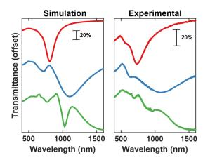
**Fig. 4** Comparison of the simulated and experimental transmittance spectra of the fabricated nanoplasmonic films. In the simulated spectra, the gold nanocups were embedded within a PMMA matrix for: 90 nm/180 nm (red), 210 nm/310 nm (blue), and 450 nm/580 nm (green) diameter/spacing structures. The experimental spectra correspond to representative spectra of gold nanocups with average diameters of 90 nm (red), 210 nm (blue), and 450 nm (green).
