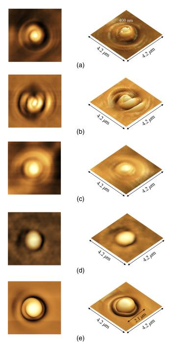
**Fig. 16** Chiral surface relief formed on the azopolymer film. (a) Right-handed-, (b) linearly- and (c) left-handed polarized 532-nm light for an exposure time of 10 min. (d) Right-handed circularly polarized light was irradiated on the device without Au thin film. (e) Original chiral surface relief in azopolymer film formed using a focused right-handed circularly polarized 532-nm optical vortex. Reproduced with permission.<sup>55</sup> Copyright 2018, The Optical Society.
