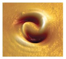
**Fig. 8** Shallow "spiral relief." The 3D image of the surface relief created on an azopolymer thin film by illumination of an orbital AM beam with  $\ell = 10$ . Reproduced with permission.<sup>56</sup> Copyright 2012, Springer Nature.
