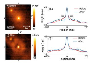
**Fig. 15** Surface reliefs (a) before and (b) after induction by a plasmonically enhanced near-field in the vicinity of a 50-nm Au nanoparticle covered by an azopolymer on a glass substrate. White arrows indicate the light polarization. (c), (d) Line plots of the surface reliefs along *X* and *Y* directions. Reproduced with permission.<sup>84</sup> Copyright 2017, Elsevier.
