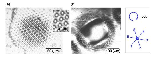
**Fig. 12** Multiple surface reliefs fabricated by an interference pattern of six circularly polarized laser beams: (a) P = 35.8 mW and  $\Delta t = 6.0$  s, (b) P = 71.6 mW and  $\Delta t = 10.0$  s. Reproduced with permission.<sup>78</sup> Copyright 2018, Springer Nature.
