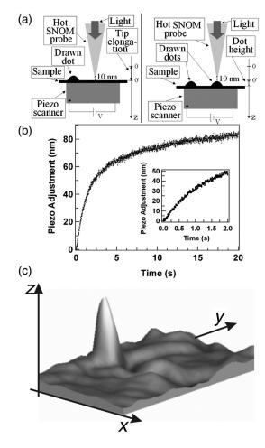
**Fig. 14** Light-injected near-field optical microscope probe scanned on the azopolymer film. (a) Schematic of the data acquisition procedure. (b), (c) A dot is formed on the film surface. The dot height is about 65 nm and the diameter is of about 200 nm. Reproduced with permission.<sup>82</sup> Copyright 2008, Wiley.
