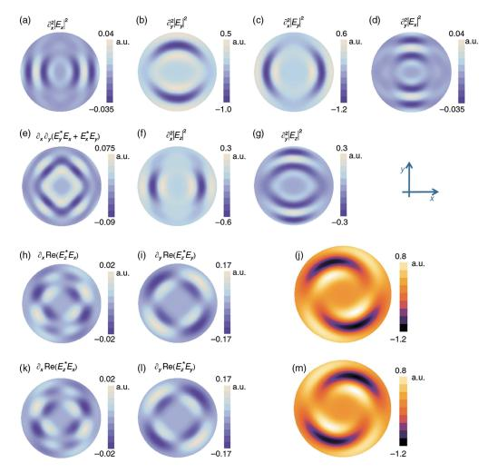
**Fig. 9** Surface reliefs calculated by theoretical models. (a)–(i), (k), (l) Surface reliefs corresponding to the various terms appearing in our model. (j), (m) Surface reliefs obtained by combining all terms at the topological charges of  $\pm 5$ . Reproduced with permission.<sup>56</sup> Copyright 2012, Springer Nature.
