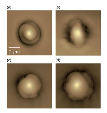
**Fig. 10** Helical surface relief with a micron-scale depth. (a) and (b) Surface reliefs formed by irradiation of orbital AM beam with J = 2 ( $\ell = 1$ , s = 1) and J = 2 ( $\ell = 2$ , s = 0) respectively. (c), (d) Surface reliefs formed by orbital AM beam with J = 0 ( $\ell = 1$ , s = -1) and J = 0 ( $\ell = -1$ , s = 1), respectively. Reproduced with permission.<sup>52</sup> Copyright 2014, Springer Nature.
