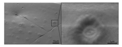
**Fig. 17** SEM images of the surface relief profile on the azopolymer layer deposited on the inner surface of the hyperlens. Reproduced with permission.<sup>86</sup> Copyright 2018, SPIE.
