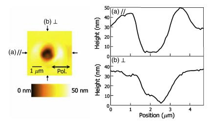
**Fig. 13** Two-photon absorption-induced surface relief formed on an azopolymer film by irradation of 920-nm femtosecond laser. (a), (b) Line plots of the relief along the parallel and perpendicular direction to light polarization. Reproduced with permission.<sup>81</sup> Copyright 2008, The Optical Society.
