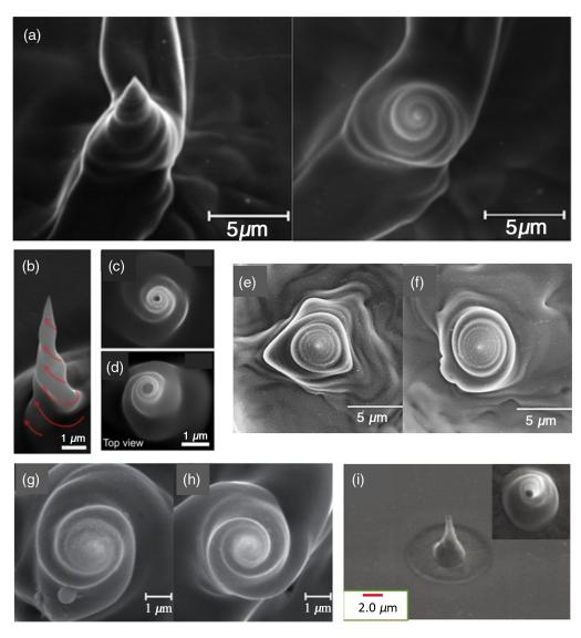
**Fig. 1** Twisted needles fabricated on various metal substrates. (a) Ta substrate.<sup>16</sup> (b)–(d) Ag film,<sup>20</sup> (e), (f) Si substrate,<sup>21</sup> (g), (h) Cu needles,<sup>29</sup> and (i) Au thin film.<sup>30</sup> Reproduced with permission.<sup>16,20,21,29,30</sup> Copyright 2012, 2017, 2016, 2017, American Chemical Society, The Optical Society, Springer Nature, Institute of Physics, Japan Laser Processing Society.
