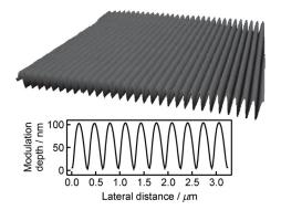
**Fig. 5** Atomic force microscopy image (top) and surface profile of relief patterns in an azopolymer film (bottom) with a period of 320 nm and surface-modulation depth of 100 nm. Reproduced with permission.<sup>61</sup> Copyright 2011, Wiley.
