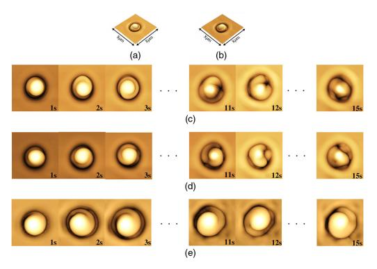
**Fig. 11** Helical surface reliefs formed by (a) right- and (b) left-handed circularly polarized Gaussian beam illumination. Temporal evolution of the (c) right- and (d) left-handed surface relief formation. (e) Right-handed helical surface relief formation formed by illumination of circularly polarized orbital AM beam with J = 2. Reproduced with permission.<sup>54</sup> Copyright 2017, The Optical Society.
