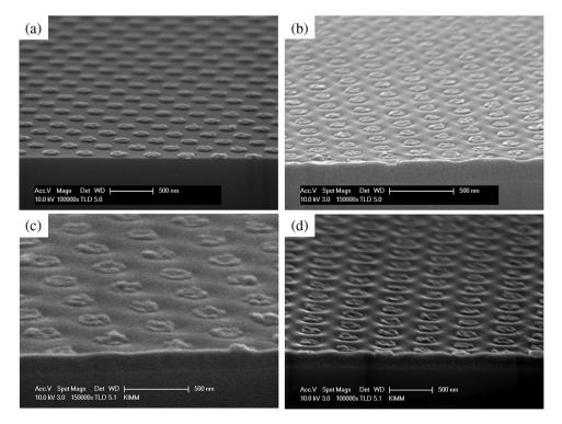
**Fig. 3** The SEM images of Ag hexagonal nanoarrays (a) protruding dot-shaped Ag nanopattern with 200-nm-diameter structures, and (b)–(d) the embedded configuration with 150-, 200-, and 265-nm-diameter structures, respectively.
