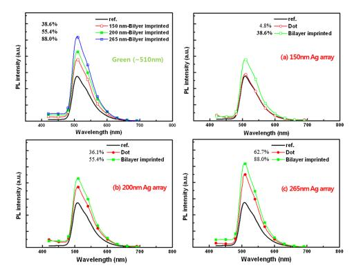
**Fig. 6** Photoluminescence (PL) enhancements with green-emitting PL materials  $[Ir(mppy)_3]$  on SiOx-deposited silver-nanopatterned glass subtrates: (a) the dependence of PL on the size of the embedded Ag nanoarray, and (b)–(d) comparisons of protruding dot-shaped Ag nanoarrays (200-nm diameter) and embedded Ag nanoarrays with diameters of 150, 200, and 265 nm, respectively.
