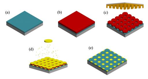
**Fig. 1** Schematic diagram of the bilayer hybrid nanoimprint (NI) process for fabricating embedded metal nanopatterns. The process consists of (a) coating the substrate with an ultraviolet (UV)-curable resist, (b) coating the substrate with a thermal NI resist, (c) thermal NI followed by UV exposure, (d) evaporation of Ag, and (e) lift-off of Ag metal and thermal NI resist.
