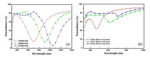
**Fig. 5** Transmittance spectra of Ag nanoarrays with 150-, 200-, and 265-nm configurations: (a) dot-shaped protruding Ag nanoarrays and (b) embedded Ag nanoarrays fabricated using bilayer hybrid NI.
