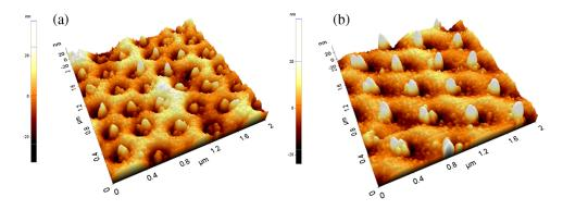
Fig. 4 Atomic force microscopy profile images of embedded Ag nanoarrays with (a) 200- and (b) 265-nm-diameter structures.
