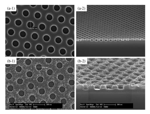
**Fig. 2** Scanning electron microscopy (SEM) images of the bilayer hybrid NI process corresponding to (a) the thermal NI and UV exposure step depicted in Figs. 1(c) and 1(b) the Ag evaporation step depicted in Fig. 1(d).
