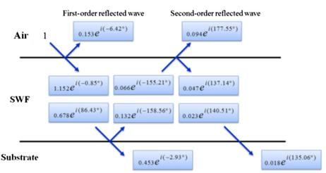
Fig. 5 Wave tracing for SWF normally illuminated by light with an electric field amplitude of unity for SWF-A at a wavelength of 676 nm and SWF-C at a wavelength of 476 nm.
