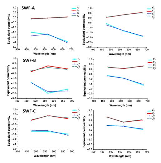
Fig. 4 Measured values of  $\varepsilon_j$  and  $\mu_j$  for SWF-A, SWF-B, and SWF-C.
