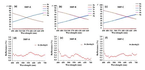
**Fig. 2** Measured spectra of the  $T_j$ ,  $R_j$ , and  $A_j = 1 - (R_j + T_j)$ ,  $j \in \{x, y\}$  of (a) SWF-A, (b) SWF-B, and (c) SWF-C and the average reflectance spectra of (d) SWF-A, (e) SWF-B, and (f) SWF-C. Light was normally incident for transmittance measurements, yet obliquely incident at 5 deg to the normal for reflectance measurements.
