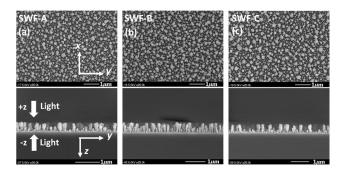
**Fig. 1** Top view and cross-sectional scanning electron microscopic images of three  $AI - SiO_2 - AI$  nanosandwich films (SWFs) with total thicknesses of (a) 420 nm, (b) 450 nm, and (c) 480 nm, respectively.
