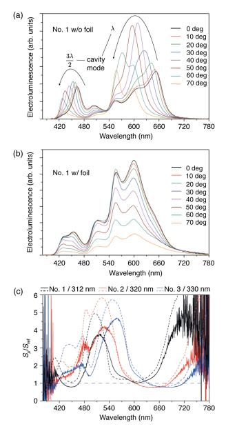
**Fig. 7** Emitted electroluminescence spectra as a function of angle of observation for devices (a) without and (b) with attached microlens array (MLA). (c) The spectral outcoupling factor of the MLA with respect to the device without MLA. In the green part of the visible spectrum, the MLA strongly contributes to the outcoupling of trapped waveguided modes, which are suppressed in the reference device [cf. (a)]. (Reproduced with permission, courtesy of American Chemical Society.)<sup>70</sup>
