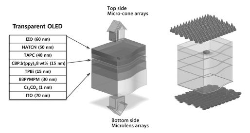
**Fig. 3** Structure of a transparent OLED with attached micro-cones proposed by Kim et al. that is designed to have minimum plasmonic losses and to achieve efficient extraction of light from waveguided modes. These OLEDs can be 2.6-fold more efficient than the respective reference device. However, the concept has only been used for monochrome OLEDs so far. (Reproduced with permission, courtesy of John Wiley and Sons.)<sup>53</sup>
