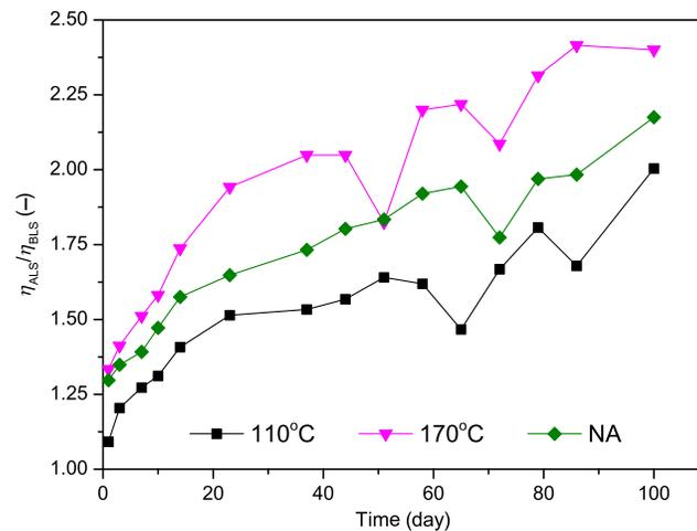
**Fig. 6** Efficiency measured after 10-min LS divided by efficiency measured before LS as a function of time for annealed at 110°C (black squares), 170°C (purple downward triangles), and for NA (green diamonds) samples. Each point is an average of five to six solar cells ALS divided by average BLS.
