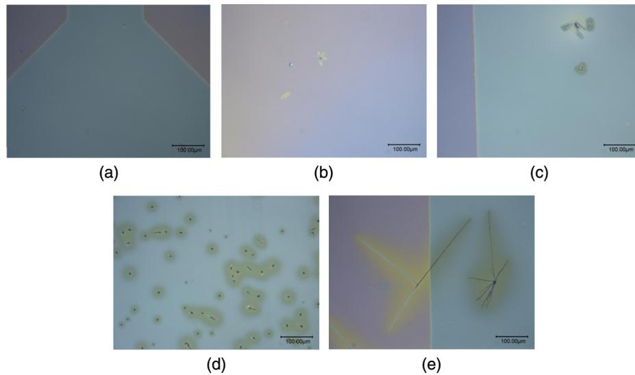
**Fig. 2** Optical images of P3HT:PCBM surfaces (a) NA and annealed at various temperatures (b) 110°C, (c) 130°C, (d) 150°C, and (e) 170°C. Lines in the images (a), (c), and (e) show the edges of ITO/glass.
