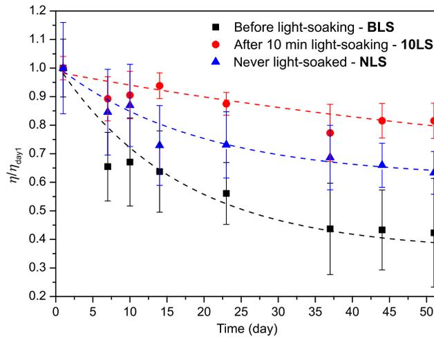
**Fig. 7** Efficiency decays for samples measured before LS (black squares), after 10 min LS (red circles), and for a sample never exposure for light-soaking illumination (blue triangles). Both groups of samples were annealed at 130°C. Each point is an average of five to six solar cells divided by average at first measurement day.
