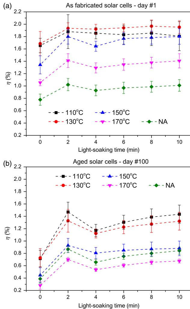
**Fig. 4** Efficiency as a function of light-soaking time for (a) fabricated and (b) aged OSCs annealed at various temperatures (each point is an average of five to six solar cells, dashed lines are guide to the eye).
