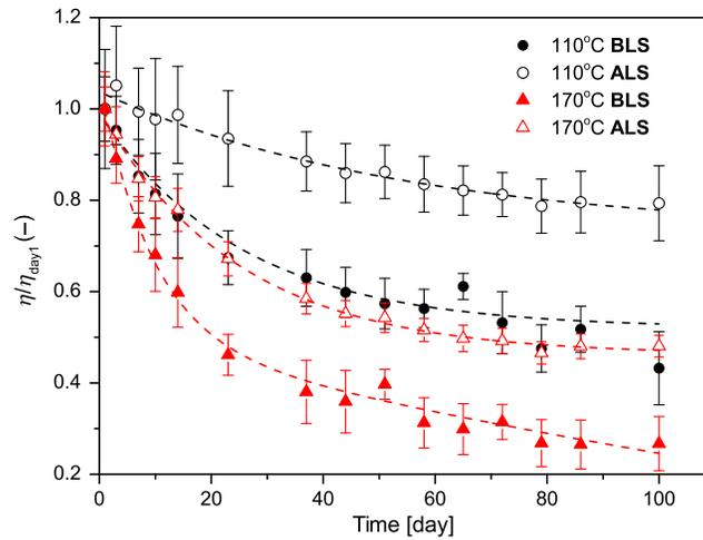
**Fig. 5** Efficiency decay for samples annealed at 110°C (black) and 170°C (red) measured before (solid circle and solid upward triangles) and after 10 min LS (open circle and open upward triangles). Each point is an average of five to six solar cells divided by average at first measurement day.
