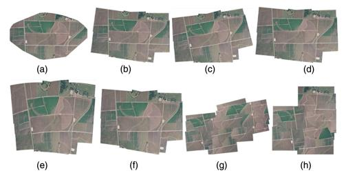
**Fig. 3** Mosaicked images from 15 images captured in four flight lines within the yellow box shown in Fig. 1 (site 2) using (a) Pix4Dmapper, (b) Autostitch, (c) Photoshop-auto, (d) Photoshop-spherical, (e) Photoshop-cylindrical, (f) Photoshop-perspective, (g) Photoshop-collage, and (h) Photoshop-reposition.
