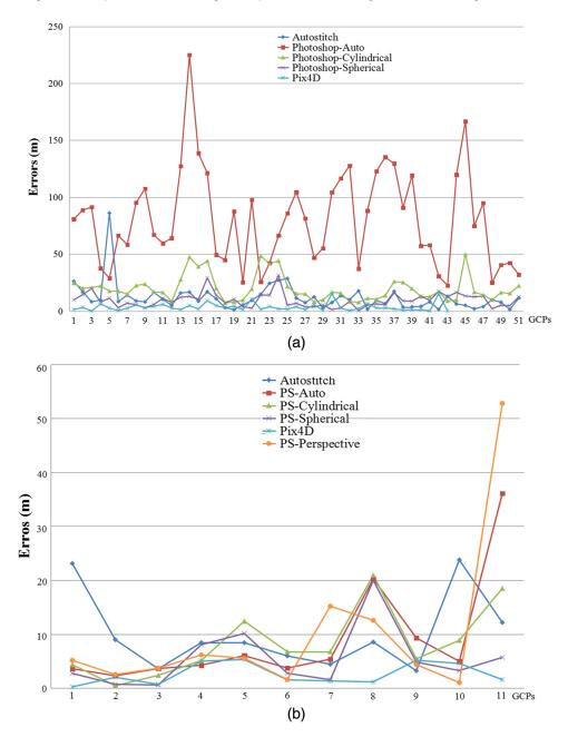
Fig. 6 Accuracy assessment results of georeferenced mosaics by different image mosaicking methods for (a) site 1 with 51 GCPs and (b) site 2 with 11 GCPs.
