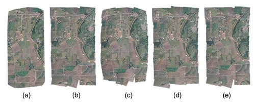
Fig. 4 Georeferenced mosaics for site 1 using (a) Pix4Dmapper, (b) Autostitch, (c) Photoshopauto, (d) Photoshop-spherical, and (e) Photoshop-cylindrical.
