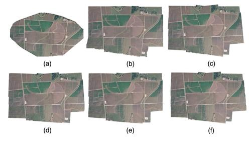
Fig. 5 Georeferenced mosaics for site 2 using (a) Pix4Dmapper, (b) Autostitch, (c) Photoshopauto, (d) Photoshop-spherical, (e) Photoshop-cylindrical, and (f) Photoshop-perspective.
