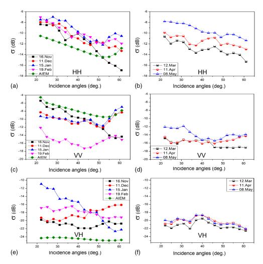
**Fig. 4** Backscattering coefficients varying with incidence angles before the heading stage (left column) and after the heading stage (right column): first row-HH, second row-VV, and third row-VH; (a), (c), (e) before the heading stage and (b), (d), (f) after the heading stage.
