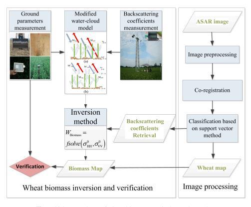
Fig. 6 Main procedures of wheat biomass monitoring and mapping.
