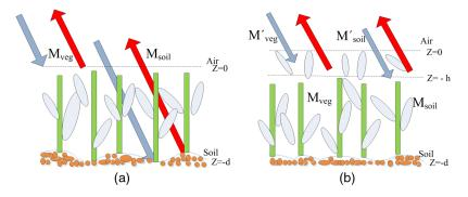
Fig. 5 Mechanism of semiempirical model: (a) water-cloud model and (b) modified water-cloud model.
