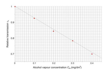
Fig. 6 Relative transmission  $\tau_a$  in function of alcohol concentration.
