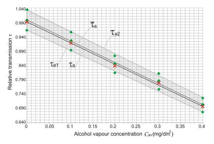
Fig. 7 Relative alcohol transmission  $\tau_a$  in function of  $C_{av}$ .
