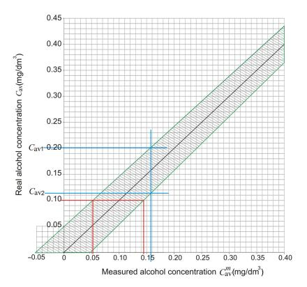
Fig. 8 Illustration of the possibility of stand-off measurement of the real value of alcohol vapor concentration in car cabins.
