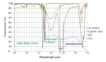
**Fig. 2** Spectral characteristics of car windowpane (Pilkington), CO<sub>2</sub>, H<sub>2</sub>O, alcohol, and lasers operating at 3.39-, 1.5-, 3.45-, and 3.59- $\mu$ m wavelengths.
