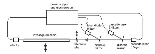
Fig. 5 Experimental setup for the investigation of relative transmission of alcohol in the cabin.
