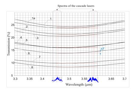
**Fig. 3** Spectral characteristics of car windowpanes: 1, windowpane of 2-mm thickness; 2, tampered Pilkington car windowpane of 3.15-mm thickness; 3, not tempered Pilkington car windowpane of 3.15-mm thickness; 4, windowpane of 2.9-mm thickness; 5, dimmed tampered Pilkington car windowpane of 3.15-mm thickness; 6, windowpane of 3.9-mm thickness; 7, dimmed tampered Soliver car windowpane of 4-mm thickness; 8, windowpane of 4-mm thickness; 1a, steamed up windowpane 1.
