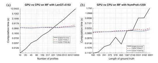
**Fig. 6** The performance of MF computing based on various libraries and processor usage. (a) Time latency used versus number of pulses, while length of data is fixed to 5162 sample points. (b) Time latency used versus length of range profile, while number of pulses is fixed to 1259.
