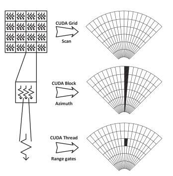
Fig. 2 The hierarchy of CUDA abstract architecture and related radar PPI scan.
