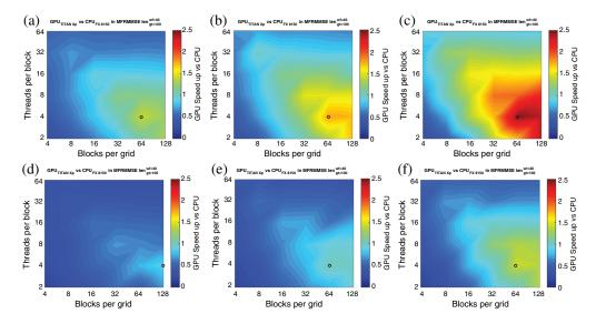
**Fig. 13** The performance comparison of MF-RMMSE between GPU and CPU implementations with various CUDA configurations and length of waveforms when length of ground truth is fixed to 100 sample points. Lengths of waveforms are from 40 to 64. The black circle represents the configuration when maximum speed up is achieved under current data format. (a)–(c) TITAN Xp, len\_wf = 40, 51, 64 and (d)–(f) TITAN Z, len\_wf = 40, 51, 64.
