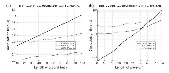
**Fig. 11** The performance comparison of MF-RMMSE based on GPU and CPU platforms. Length of (a) waveform = 51 and (b) ground truth = 100.
