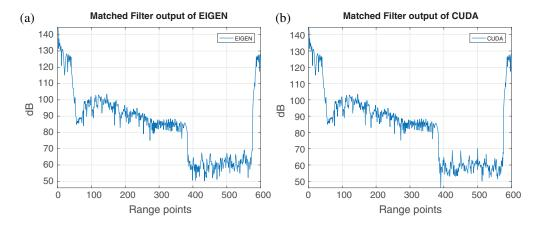
Fig. 15 Averaged output results of pulse compression implementation using NASA's HIWRAP radar data. Averaged MF output of (a) EIGEN and (b) CUDA.
