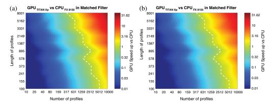
**Fig. 7** The performance comparison of MF based on GPU and CPU platforms. (a) TITAN Xp and (b) TITAN Z.
