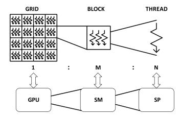
Fig. 5 The hierarchy of CUDA abstract architecture and related GPU physical architecture.
