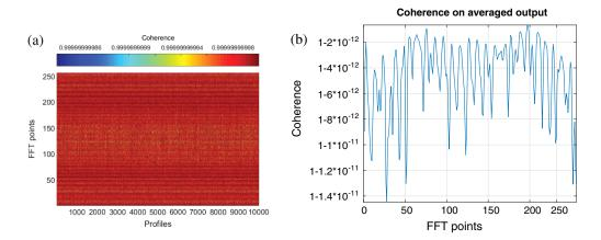
Fig. 17 Coherence results of pulse compression implementation using NASA's HIWRAP radar data. Magnitude-square coherence estimate between (a) EIGEN and CUDA outputs and (b) averaged EIGEN and CUDA outputs.
