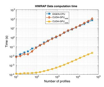
Fig. 18 Time consumption of CPU and GPU versus number of range profiles handling in HIWRAP data, whereas GPU time consumption without data transfer is demonstrated separately.
