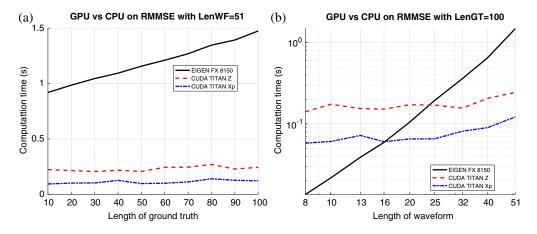
**Fig. 8** The performance comparison of RMMSE based on GPU and CPU platforms. Length of (a) waveform = 51 and (b) ground truth = 100.
