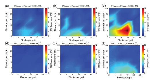
**Fig. 10** The performance comparison of RMMSE between GPU and CPU implementations with various CUDA configurations and length of waveforms when length of ground truth is fixed to 100 sample points. Lengths of waveforms are from 32 to 51. The black circle represents the configuration when maximum speed up is achieved under current data format. (a)–(c) TITAN Xp, len\_wf = 32, 40, 51 and (d)–(f) TITAN Z, len\_wf = 32, 40, 51.
