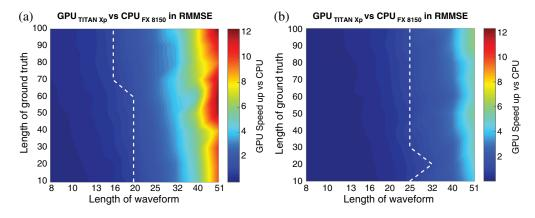
Fig. 9 The performance comparison of RMMSE based on GPU and CPU platforms. (a) TITAN Xp and (b) TITAN Z.
