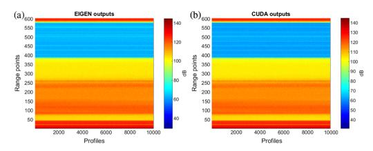
**Fig. 14** Output results of pulse compression implementation using NASA's HIWRAP radar data. MF output of (a) EIGEN and (b) CUDA.
