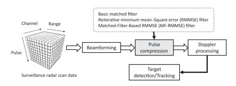
Fig. 1 The basic processing chain of pulsed-Doppler radar.
