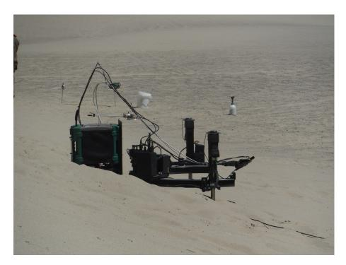
**Fig. 7** The GRIT-T as it measures the radiance reflected from a sloped sand surface. Note that the goniometric system is leveled and still able to track the same spot on the target. Also note that, on a sloped surface, the maximum zenith angle that can be reached is reduced, since the distance from the sensor to the target is enlarged.
