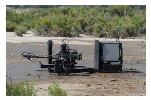
Fig. 5 The GRIT-T as it measures a "true" 70-deg zenith angle with respect to the target. Here, the GRIT-T pointing head is counter-rotated to ensure that the same spot on the target is measured at each view angle position. The magnitude of this counter-rotation is determined for every zenith view angle.
