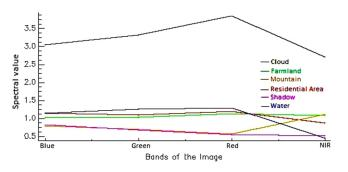
Fig. 3 Means of different objects in the study plots derived from the GF-1 image.
