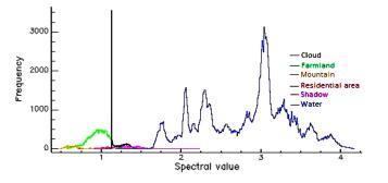
Fig. 4 Spectral curves of all six types of surface features using the green/NIR band ratio.
