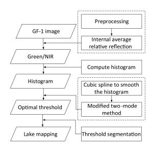
Fig. 2 Flowchart showing the overall procedure of the methods proposed in this study.
