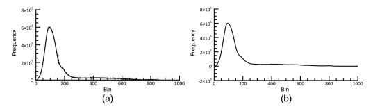
Fig. 5 Histogram of the band ratio (a) before and (b) after cubic spline interpolation.
