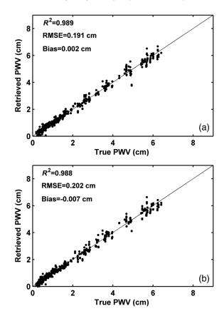
Fig. 12 The scatter plots of the retrieved and true PWV by model 4. (a) SRF2 and (b) SRF3.
