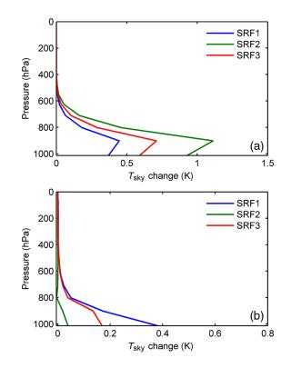
**Fig. 7**  $T_{sky}$  change for SRFs 1 to 3 due to 5% and 1 K increasing in the water vapor mixing ratio (a) and temperature (b) profile at different pressure level for the MLS atmosphere.
