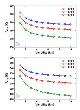
Fig. 10 The relationship between  $T_{sky}$  (urban aerosol model) with VIS for different SRFs. (a) MLS and (b) MLW atmosphere.
