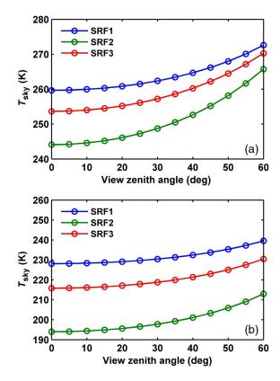
Fig. 11 The relationship between  $T_{sky}$  (urban aerosol model, VIS = 5 km) with VZA for different SRFs. (a) MLS and (b) MLW atmosphere.
