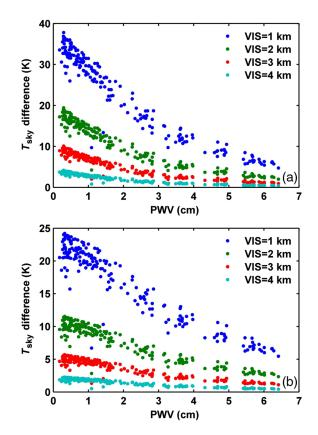
**Fig. 8** The  $T_{sky}$  change between different VIS (1 to 4 km) and MODTRAN default urban aerosol extinction model (VIS = 5 km) vary with PWV. (a) SRF2 and (b) SRF3.
