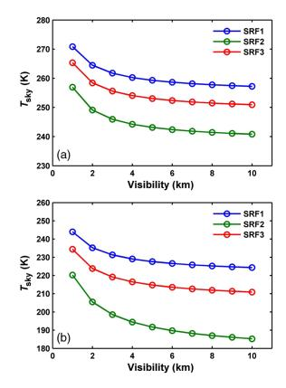
Fig. 9 The relationship between  $T_{sky}$  (rural aerosol model) with VIS for different SRFs. (a) MLS and (b) MLW atmosphere.
