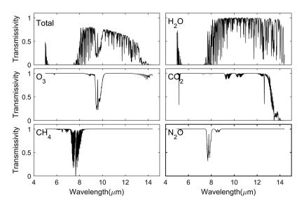
Fig. 1 Atmospheric transmittances of various absorbing gases calculated by the MODTRAN 5.2 for the standard MLS atmosphere in 5.0 to 14.5  $\mu$ m.
