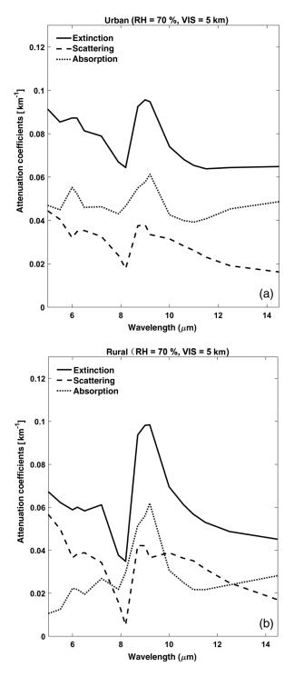
Fig. 4 Attenuation coefficients for (a) urban and (b) rural aerosol at 70% RH.
