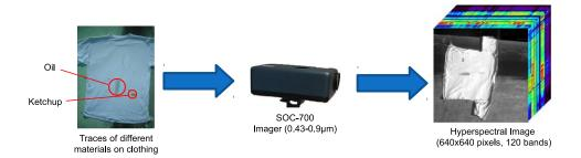
Fig. 6 Phantom image generation for the experiments: a hyperspectral image of a scene simulating traces of different materials on clothing was collected using a SOC-700 imager.
