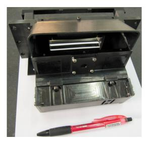
Fig. 1 Picture of the multispectral line scanner.
