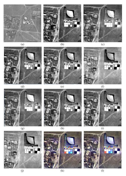
**Fig. 7** An example by registering an image captured by an array camera onboard. (a) Whole image from array camera, (b) subregion of (a), (c) blue band, (d) green band, (e) red band, (f) near-infrared band, (g) registered blue band, (h) registered green band, (i) registered red band, (j) registered near-infrared band, (k) true color image (before), and (l) after registration.
