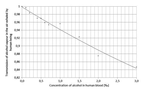
**Fig. 4** Transmission of alcohol vapor in the air exhaled by a human being in function of concentration of alcohol in blood.
