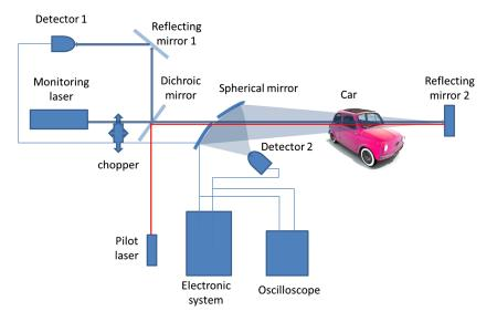
Fig. 1 Experimental setup for detection of alcohol in cars.
