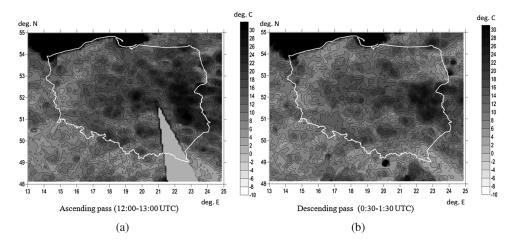
**Fig. 7** Spatial distribution of Tb18V–Tb18H difference for the area of Poland on April 10, 2013. High values in the eastern and central part of Poland are well related to intensive snow melting connected with flood in this region, (a) ascending pass and (b) descending pass.
