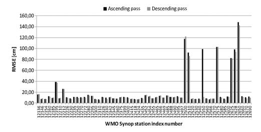
Fig. 3 Comparison of snow depth measured at the ground and retrieved from GCOM-W1 data— RMSE [cm] for individual Synop stations.
