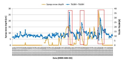
**Fig. 6** Melting snow detection (red boxes indicate snow melt periods)—depletion of snow cover connected with significant peaks of Tb18V–Tb18H temperature difference. Presented example concerns Koło Synop station (WMO index number 12345).
