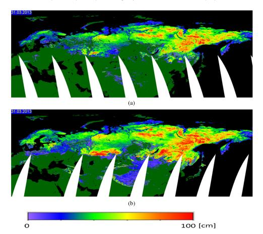
**Fig. 5** Comparison of GCOM-W1 snow depth for the area of Euro-Asia on the same day: (a) ascending passes above and (b) descending passes below.
