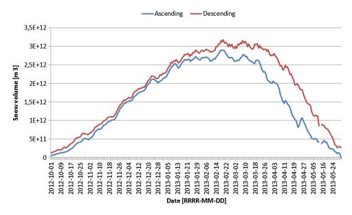
**Fig. 4** Snow volume calculated from GCOM-W1 snow depth product, for the part of Northern Hemisphere (20 deg–85 deg N, 0 deg–360 deg E).
