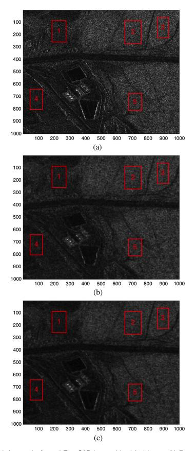
Fig. 5 Simulation results for real TerraSAR image: (a) original image, (b) filtered image via MinBAD approach, and (c) filtered image via unbiased-average MinBAD approach.
