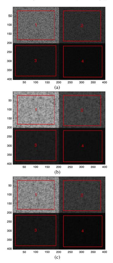
**Fig. 3** Simulation results for artificial scene synthetic aperture radar (SAR) image: (a) original image, (b) filtered image via MinBAD approach, and (c) filtered image via unbiased-average MinBAD approach.
