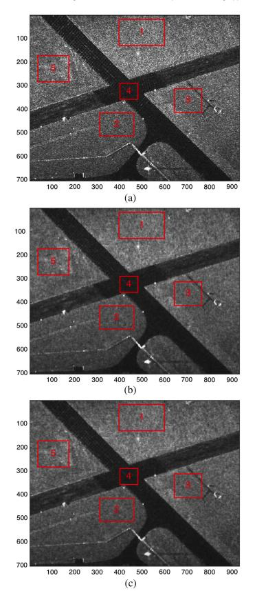
Fig. 4 Simulation results for real SAR image: (a) original image, (b) filtered image via MinBAD approach, and (c) filtered image via unbiased-average MinBAD approach.
