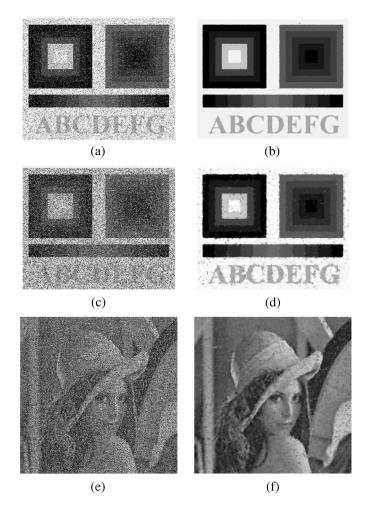
**Fig. 1** Denoise results by minimum biased diffusion (MinBAD) method: (a) image with 10% additional noise (PSNR = 15.61 dB); (b) denoised image (PSNR = 34.31 dB, three iterations); (c) image with 50% additional noise (PSNR = 8.60 dB); (d) the denoised image (PSNR = 26.92 dB, five iterations); (e) Lena image with 60% additional noise (PSNR = 11.47 dB); and (f) the denoised Lena image (PSNR = 24.07 dB, five iterations).
