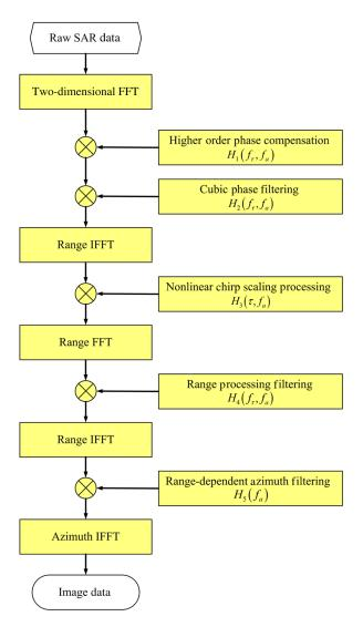
Fig. 3 Block diagram of the proposed higher order imaging algorithm.
