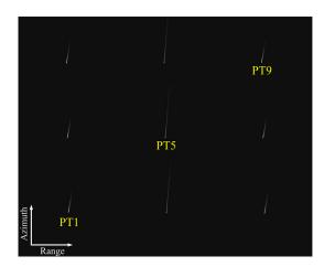
Fig. 9 Focused result by the NLCS algorithm.
