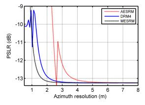
Fig. 7 Peak sidelobe ratio (PSLR) as a function of azimuth resolution.
