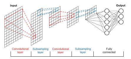
Fig. 2 The common structure of convolutional neural network.
