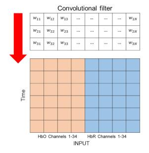
**Fig. 6** The input data consisted of the concentration changes of HbO (red) and HbR (blue) overall channels. A convolutional filter ran through the input data along the vertical axis.
