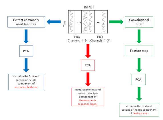
**Fig. 7** The overall procedure to visualize signal features, including the hemodynamic response signal, commonly used features in fNIRS-based BCI, and output of the convolutional filter (feature map). The first and second principle components of the signal features are illustrated for the visualization.
