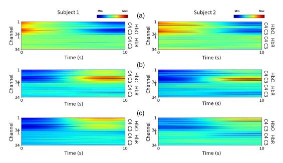
Fig. 8 Average hemodynamic response of each execution task measured from subject 1 and 2: (a) rest, (b) right-, and (c) left-hand motor execution. Each input presents concentration changes of HbO and HbR overall 34 channels. Red and blue colors represent the maximum and minimum amplitude, respectively.
