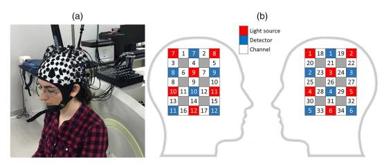
**Fig. 4** (a) A subject with optodes over motor area C3 and C4 based on the international 10–20 system and (b) the source and detector configuration. Channel numbers 1 to 17 and 18 to 34 were placed over motor areas C4 and C3, respectively.
