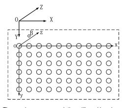
Fig. 6 The moving camera and the still workbench coordinate systems.
