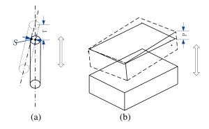
Fig. 5 The impact on perpendicularity caused by Z-axis movement.
