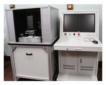
Fig. 1 Video-based inspecting instrument for watch escapement (VIIWE).
