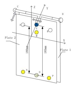
Fig. 7 The adjustment mechanism for perpendicularity.
