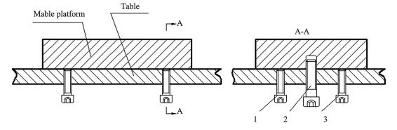
Fig. 8 Parallelism adjustment sketch.
