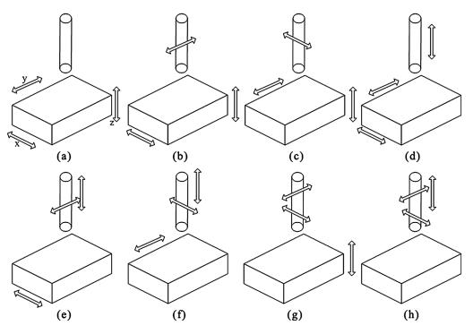
Fig. 2 Eight types of movement layout for linear 3-D motion.
