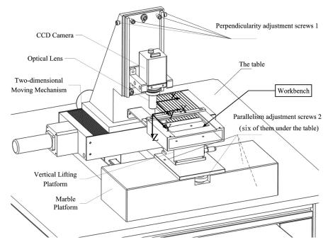
Fig. 9 Main structure of VIIWE.
