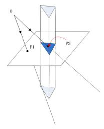
Fig. 3 Illustration of how to determine whether the intersection is within the triangle in the proposed method.
