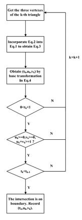
Fig. 1 Flowchart of the ray-triangle-based method.
