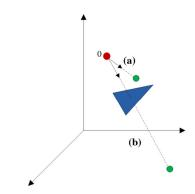
**Fig. 2** The photon migration within a limited step. (a) The photon which does not intersect with the triangle in the next step of migration. (b) The photon which intersects with the triangle during the next step of migration.
