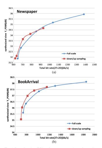
Fig. 4 Rate distortion (RD) performance comparison of encoding depth maps between full scale and down/upsampling based method. (a) Book Arrival and (b) Newspaper.
