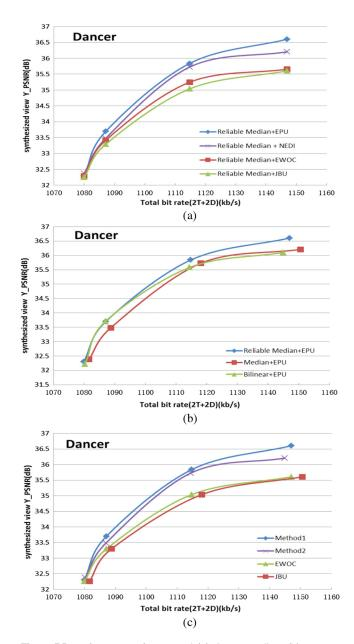
Fig. 5 RD performance of proposed (a) downsampling, (b) upsampling, and (c) down/upsampling method.
