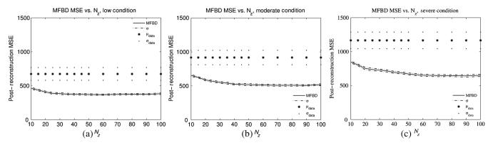
Fig. 5 Mean square error (MSE) versus number of Zernike coefficients. With the number of frames held constant at 50, the number of Zernike coefficients are varied from 10 to 100 for (a) low condition  $C_N^2=2.25\times 10^{-14}~{\rm m}^{(-2/3)}$ , (b) moderate condition  $C_N^2=3.75\times 10^{-14}~{\rm m}^{(-2/3)}$ , and (c) severe condition  $C_N^2=5.25\times 10^{-14}~{\rm m}^{(-2/3)}$ .
