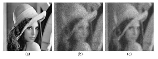
Fig. 13 Case 1 sample images, mean photon rate  $2 \times 10^6$ ,  $C_N^2 = 2.25 \times 10^{-14}$  m $^{(-2/3)}$ . Compares the (a) diffraction-limited image with (b) a single sample image and (c) a sample reconstructed object.
