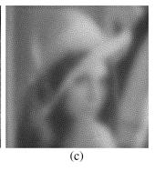
Fig. 17 Case 3 sample images, mean photon rate  $2 \times 10^6$ ,  $C_N^2 = 5.25 \times 10^{-14} \text{ m}^{(-2/3)}$ . Compares the (a) diffraction-limited image with (b) a single sample image and (c) a sample reconstructed object.
