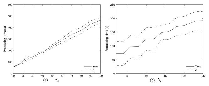
Fig. 4 Processing time versus number of Zernike terms (a), and number of frames used in reconstruction (b).
