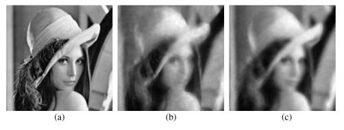
Fig. 8 Case 2 sample images. Compares the (a) diffraction-limited image with (b) the single sample image and (c) a sample reconstructed object.
