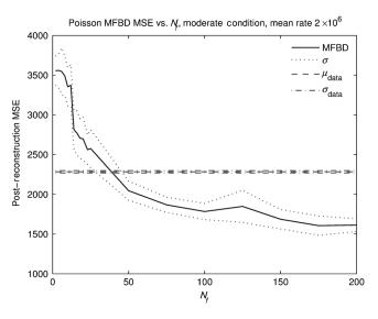
**Fig. 15** MSE versus number of frames. Poisson case 2 moderate turbulence  $C_N^2=3.75\times 10^{-14}~{\rm m}^{(-2/3)}$ , mean photon rate  $2\times 10^6$ .
