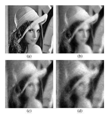
**Fig. 1** Horizontal imaging simulator output. Single image representative samples of the horizontal image simulator output: (a) diffraction-limited image, (b) image for  $C_N^2 = 2.25 \times 10^{-14} \ \mathrm{m}^{(-2/3)}$ , (c) image for  $3.75 \times 10^{-14} \ \mathrm{m}^{(-2/3)}$ , and (d) image for  $5.25 \times 10^{-14} \ \mathrm{m}^{(-2/3)}$ .
