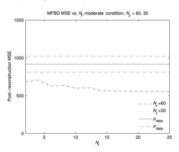
**Fig. 9** MSE versus number of frames. Case 2 moderate turbulence  $C_N^2=3.75\times 10^{-14}$  with 30 and 60 Zernike terms.
