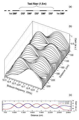
Fig. 5 A test fiber (a) composed of five single mode fibers and dispersion shifted fibers, a three-dimensional graph of Brillouin gain spectra (b) and Brillouin gain variations at the fixed Brillouin frequencies according to the distance (c).
