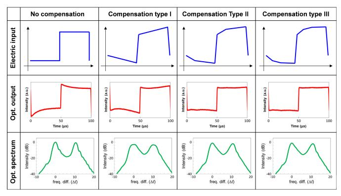
Fig. 2 Four different types of electrical input waveforms (the first row) into a laser diode (LD) for generating two time-divided lightwaves and their optical output powers (the second row) and spectra (the third row).
