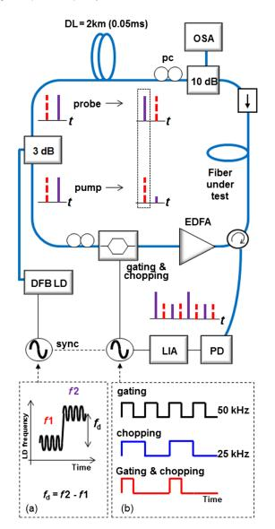
**Fig. 1** The schematic of the experiment setup with a modulated input function (a), and a gating and chopping function (b). A distributed feedback laser diode (DFB LD), lock-in-amplifier (LIA), and optical spectrum analyzer (OSA).
