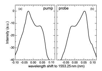
**Fig. 3** An optical spectrum (a) of a pump after a probe lightwave (b) included in a pump lightwave was eliminated by a pump gate.
