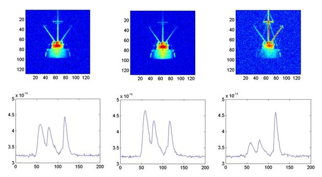
Fig. 19 Illustration of the effect of large beam jitter with an rms value equal to 1/3 of the field-of-view (FOV). The peak positions remain aunchanged but not the mutual peak amplitudes.
