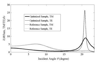
**Fig. 8** The calculated  $I(485 \text{ nm}, TM/TE)/I_0$  versus  $\theta$  of the optimized and reference samples.
