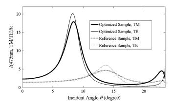
**Fig. 6** The calculated  $I(475 \text{ nm, TM/TE})/I_0$  versus  $\theta$  of the optimized and reference samples.
