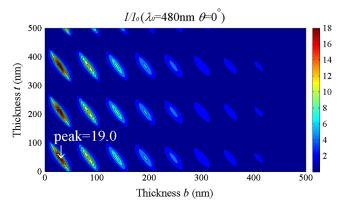
**Fig. 4** The calculated  $I(480 \,\mathrm{nm}, 0 \,\mathrm{deg})/I_0$  versus parameters t and b represented by the contour figure.
