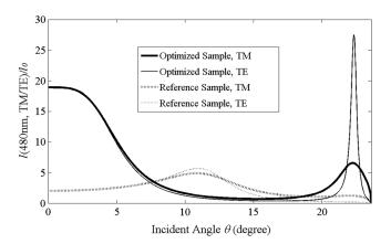
**Fig. 7** The calculated  $I(480 \text{ nm, TM/TE})/I_0$  versus  $\theta$  of the optimized and reference samples.
