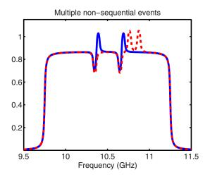
**Fig. 8** An example of a possible nonsequential BGS. It is clear from the spectrum that at least two events (local heating or strain) have taken place, but it is not readily apparent which of the two peaks (dashed line) corresponds to which location along the fiber. Tracking the BGS in time can alleviate this problem.
