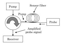
Fig. 13 Example PPS configuration.
