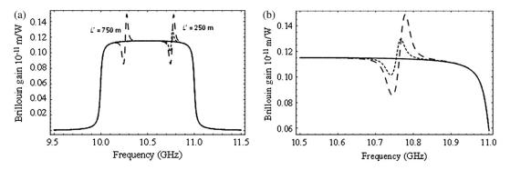
**Fig. 2** (a) Brillouin gain spectrum for the example for  $\Delta T = 0$ , 10, and 30 K, (b) expanded view in the vicinity of the thermal activity region ("anomaly"). The amplitude of the change in BGS increases with increasing temperature. Changing L' simply shifts the location of the spectral "anomaly" as illustrated with the  $\Delta T = 30$  K calculation repeated for 750 m [shown in (a)].
