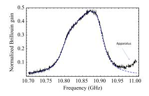
**Fig. 4** Brillouin gain spectrum of the fundamental acoustic mode of the LGF of this study (solid line). The modeling fit to the data is also shown (dashed line). The total fiber length is 16.7 m.
