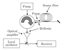
Fig. 10 Example of a CDS configuration.
