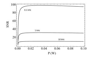
**Fig. 12** SNR of the homodyne system plotted as a function of *P* for three different electrical bandwidths  $B_N$ .
