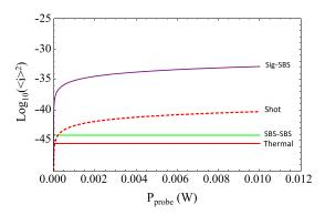
Fig. 14 Logarithm of the variances of the various identified noise sources for the PPS configuration. The variance is calculated in units of Amperes squared.
