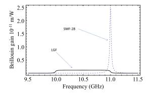
Fig. 1 Brillouin gain spectra for a conventional single mode fiber (SMF-28) and that of the longitudinally graded optical fiber (LGF).
