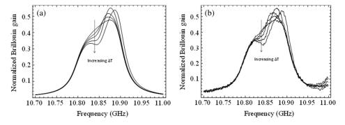
**Fig. 5** (a) Modeled BGS of the LGF at  $\Delta T = 0$ , 5, 10, 20, 40 K and L' = 9.7 m and  $\Delta L = 1.13$  m, (b) measured BGS for the same thermal conditions.
