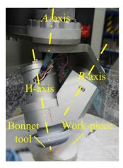
Fig. 6 Experimental prototype for bonnet polishing.
