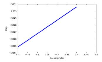
**Fig. 2** Chirp versus saturable absorption parameter  $\delta_{SA}$ .
