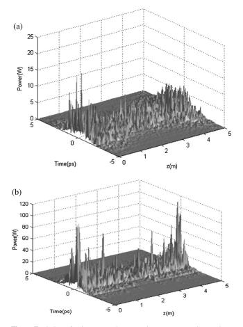
**Fig. 3** Evolution of substructure in a 5 m ring resonator when pulses grow from spontaneous emission with group-velocity dispersion: (a)  $\beta_2 = -0.014 \text{ ps}^2/\text{m}$ , (b)  $\beta_2 = -0.012 \text{ ps}^2/\text{m}$ . Other parameters are  $\gamma = 0.012 \text{ (Wm)}^{-1}$ ,  $\alpha_2 = 0.3$ ,  $T_2 = 0.047 \text{ ps}$ ,  $\alpha = 0.17823 \text{ m}^{-1}$ , and  $g = 0.78275 \text{ m}^{-1}$ .
