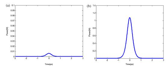
Fig. 5 Profiles of parabolic pulse at (a) z = 0.1 m and (b) z = 6 m.
