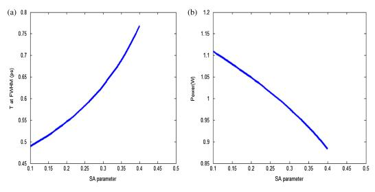
Fig. 7 (a) width of soliton and (b) output power versus  $\delta_{\rm SA}.$
