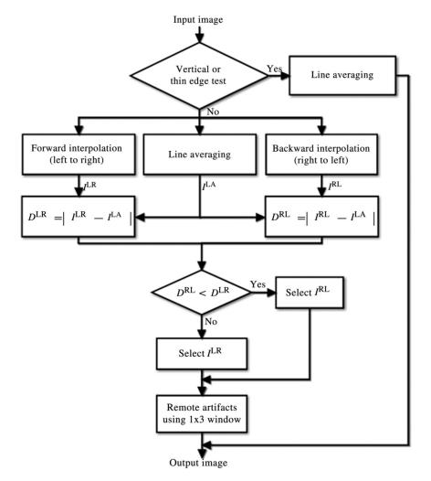
Fig. 4 Flow chart of the proposed interpolation method.
