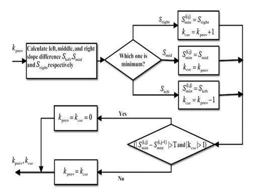
Fig. 1 Flow chart of the edge slope tracing (EST) process.
