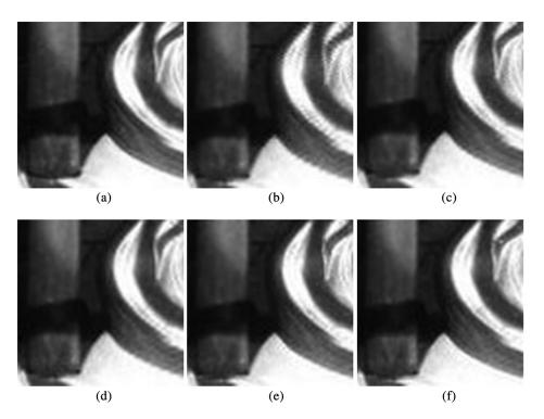
Fig. 10 Cropped regions after deinterlacing: (a) original, (b) ELA, (c) GGD, (d) LCIM, (e) MLSM, and (f) the proposed method.
