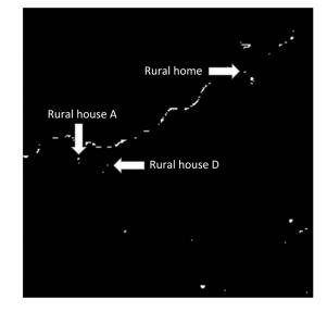
Fig. 18 Detections from processing channel 3 and 4 imagery using Eq. (41) and CFAR level of  $10^{-14}$ .
