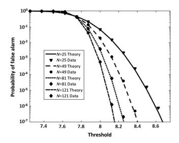
Fig. 6 Comparison of computer simulation results with probability of false alarm, Eq. (54), for N = 25, 49, 81, and 121.
