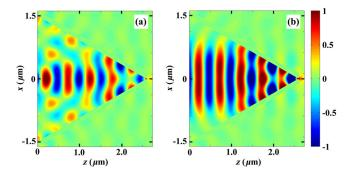
Fig. 2 Distributions of the electric field component Ex in the TMG (NA = 0.75,  $\lambda = 500$  nm, BW = 9.0 mm): (a) without and (b) with the amplitude modulation.
