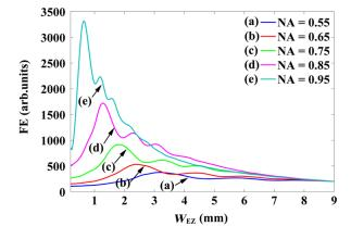
Fig. 4 FE as a function of the euphotic zone size  $W_{EZ}$  for various NAs (the other parameters are the same as those stated in Fig. 1).
