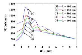
Fig. 5 FE as a function of the euphotic zone size for various incident wavelengths (the other parameters are the same as those stated in Fig. 1).
