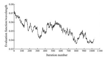
Fig. 6 Evaluation function variation curves for NA 1.2 lithographic PO.
