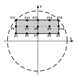
Fig. 2 Field points on the image plane.
