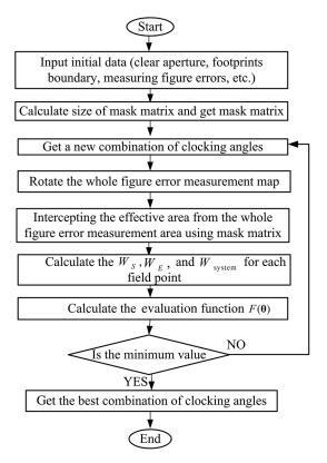
Fig. 5 Flow chart of the clocking-optimization method.
