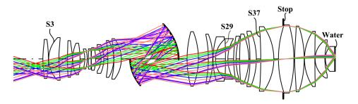
Fig. 1 Layout of NA 1.2 lithographic projection optics.
