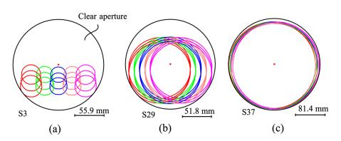
Fig. 3 Footprints of three surfaces of 15 field point of NA 1.2 projection optics (PO): (a) Surface 3, (b) Surface 29, and (c) Surface 37.
