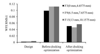
**Fig. 7** Contrastive analysis, before and after figure-error balancing, for the NA 1.2 lithographic PO.
