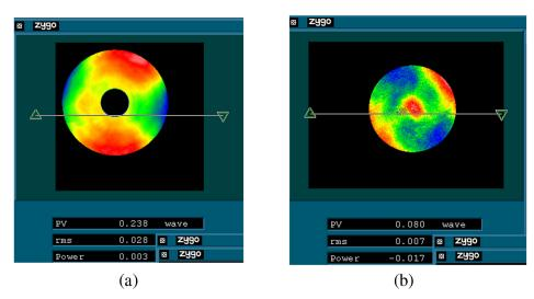
Fig. 9 Figure-error maps for the following: (a) the ring-shaped region of the front surface of L2 and (b) the central region of the back surface of L3.
