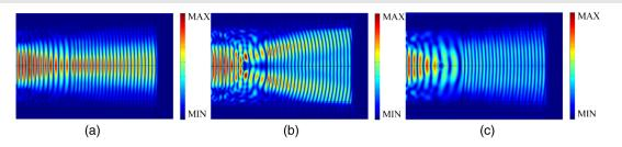
**Fig. 1** Displacement vector simulation in inhomogeneous materials. (a) Original waves without obstacle, (b) waves without cloak, and (c) waves with the designed cloak.
