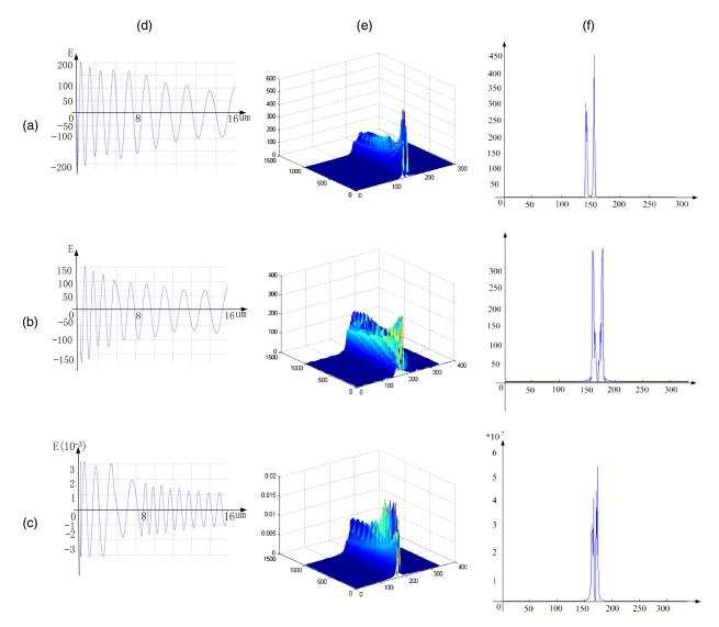
**Fig. 3** Analysis of scattering effects on directional cloaks. Horizontal: (a) without obstacles, (b) with obstacles but without cloaks, and (c) with both obstacles and cloaks. Vertical: (d) waveforms of intermediate position in the designed inhomogeneous materials; (e) 3-D diagrams of FRFT signals in (d) column, where *x*-label is the transformation angle, *y*-label is the original signal, and *z*-label is the FRFT result; and (f) matching order of FRFT results.
