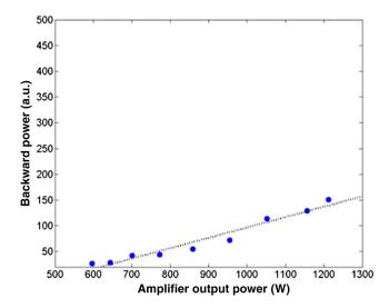
Fig. 3 Backward power versus output power for one of the NuKW amplifiers driven with a 2<sup>9</sup> – 1 PRBS pattern at a frequency of 10 GHz.
