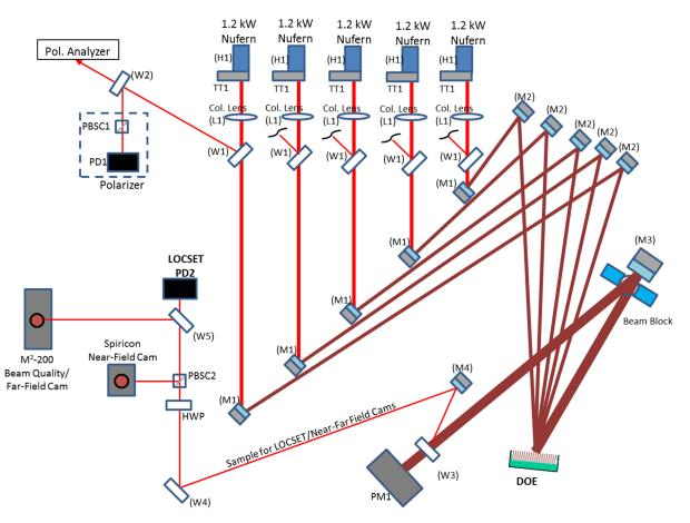
**Fig. 6** Schematic of the 1 × 5 DOE beam combining setup. After collimation, samples of each beam were used for polarization locking and a sample of the combined output beam was used for LOCSET phase locking and beam quality analysis. M1–4: reflective dielectric mirrors, W1–5: beam sampling wedges, HWP: half-wave plate, PBSC: polarizing beam splitter cube, PD1–2: photodetector, and PM1: power meter.
