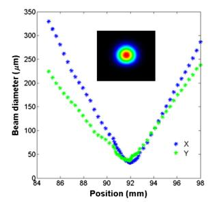
Fig. 8 Near diffraction-limited beam quality was measured with an  $M^2$  of <1.1. The inset shows the beam profile of combined output beam.
