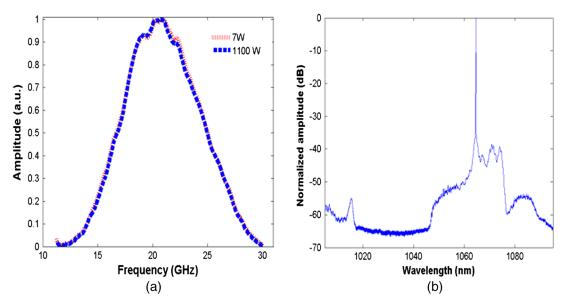
**Fig. 4** (a) FPI linewidth measurement at 7 W (red dotted) and 1100 W (blue dashed), respectively. (b) Wide-range (100 nm) forward spectrum captured by OSA at 1100 W. We note no spectral broadening was observed at high power.
