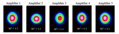
Fig. 5 Measured beam profiles for each of the NuKW amplifiers at 1100 W. All five laser beams exhibited excellent beam quality with *M*<sup>2</sup> values less than 1.1.
