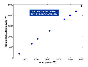
Fig. 7 Input power versus combined output power for the five-channel beam combining. An output power of 4.9 kW with 82% combining efficiency was demonstrated.
