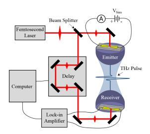
Fig. 3 Schematic diagram of the typical configuration of electro-optic sampling of THz pulses in a TDS system.
