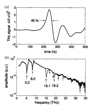
**Fig. 17** (a) The temporal THz wave form and (b) its corresponding Fourier transform amplitude spectrum (upper trace, solid line), together with spectrum measured in the presence of PTFE sample (lower trace, dotted line). Reprinted from Ref. 182, with permission of AIP Publishing.
