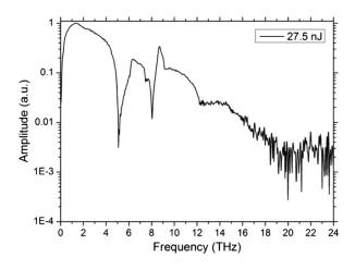
**Fig. 16** FFT amplitude as a function of frequency, showing a bandwidth approaching 20 THz. Reprinted from Ref. 135 with permission from OSA Publishing.
