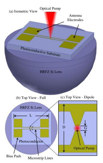
**Fig. 2** (a) Isometric view of a typical THz PCA device mounted on a HRFZ Si lens. (b) Full top view of the THz PCA and (c) expanded top view of the centrally located THz dipole structure only showing gap dimension G and dipole length D.
