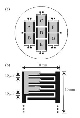
**Fig. 10** (a) Schematic of THz emitter composed of seven photoconductive antenna units having interdigitated electrode structure. The units are labeled A–G for later reference. (b) Structure of electrodes and shadow mask of each unit.<sup>130</sup> Copyright 2006 The Japan Society of Applied Physics.
