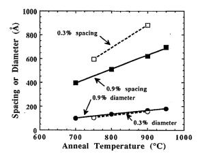
**Fig. 5** Precipitate diameter and precipitate spacing versus 30-s anneal for the two LT-GaAs films used in this study.<sup>53</sup> Reprinted from Ref. 53, with permission of AIP Publishing.
