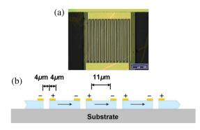
**Fig. 9** (a) Micrograph of terahertz array antenna device. (b) Crosssectional view of terahertz antenna array. Reprinted from Ref. 131, with permission of AIP Publishing.
