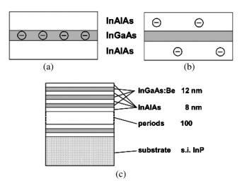
**Fig. 8** (a) Embedded photoconductor; (b) electron trapping; and (c) multilayer structure. Reprinted from Ref. 115 with permission from OSA Publishing.
