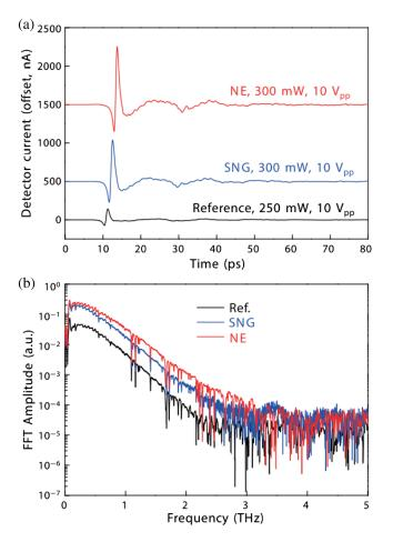
**Fig. 15** THz emission from the large-aperture PCAs: (a) time-domain curves and (b) FFT spectra. Reprinted with permission from Ref. 167 under a Creative Commons Attribution 4.0 International License.
