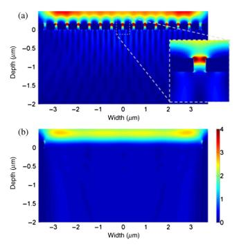
**Fig. 11** Cross-section of plasmonic enhancement showing local intensity increase. (a) PE-LT-GaAs and (b) LT-GaAs. Reprinted from Ref. **114**. Copyright 2015 American Chemical Society.
