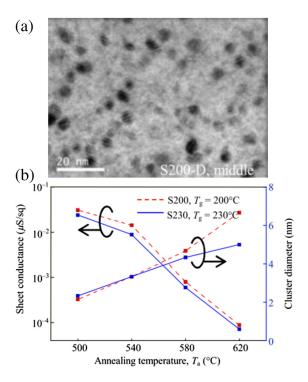
**Fig. 6** (a) TEM photograph of annealed LT-GaAs layer and (b) sheet conductance and cluster diameter as functions of annealing temperature. Reproduced from Ref. 57 with permission from the Electronics and Telecommunications Research Institute.
