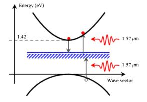
**Fig. 7** Schematic of two-step 1.57-µm photon absorption process enabled by midgap states in arsenic-rich LT-GaAs.<sup>114</sup> Reprinted with permission from Ref. 114. Copyright 2015 American Chemical Society.
