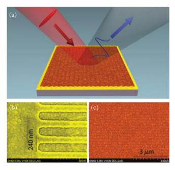
**Fig. 12** (a) Schematic diagrams of the nanostructured Au/Cu<sub>2</sub>O Schottky junction THz emitter. The pump laser pulses are incident on the sample, generating THz pulses. A nanograting is fabricated at the interface to facilitate the excitation of surface plasmons. (b, c) False-color SEM image of the grating after the deposition of Au and Cu<sub>2</sub>O, respectively. Reprinted with permission from Ref. 157. Copyright 2014 American Chemical Society.
