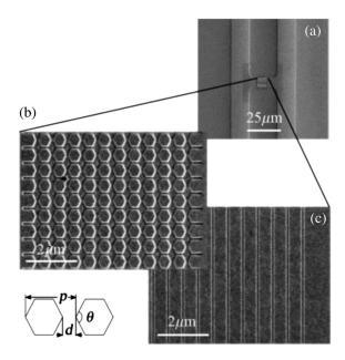
**Fig. 13** (a) SEM image of the 20- $\mu$ m dipole on SI-GaAs substrate. (b) The active area of the hexagonal plasmonic array. (c) The active area of the strip plasmonic array. The diagram shows apex angle  $\theta$ , gap size *d*, and periodicity *p*. Reprinted from Ref. 161 with permission from OSA Publishing.
