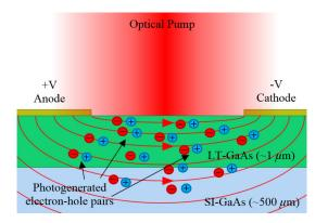
Fig. 4 Cross-section illustration of optical carrier generation at the dipole gap of a LT-GaAs based THz PCA showing the flux lines of the electric field in red arrows.
