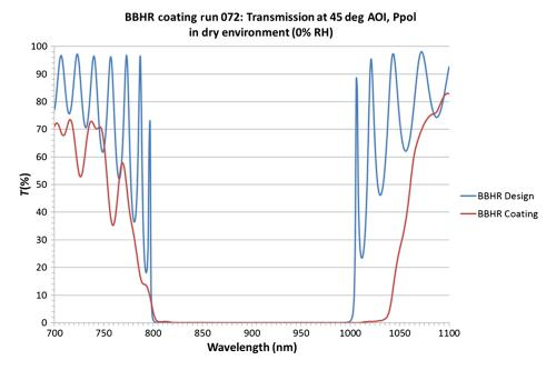
**Fig. 2** Transmission spectrum as measured under dry (0% RH) conditions at 45-deg AOI, Ppol for the BBHR coating of Run 072, shown in comparison to the coating's corresponding design transmission spectrum.
