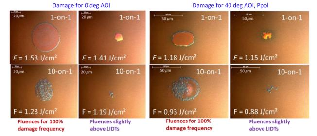
Fig. 9 Morphology images of laser-induced damage caused by 675-fs pulses at 1053 nm on the BBHR coating of Run 072 at 0-deg AOI and at 40-deg AOI, Ppol in 1-on-1 and 10-on-1 tests and with fluences as indicated.
