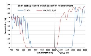
**Fig. 6** Measured transmission spectra of the BBHR coating of Run 072 at 0-deg AOI and at 40-deg AOI, PpoI, under dry (0% RH) conditions. The thick black vertical line indicates 1053 nm, the center wavelength of the CEA-CESTA 675 fs LIDT test laser pulses. It is well within the central zone of the HR band for 0-deg AOI and near the HR band edge for 40-deg AOI, PpoI.
