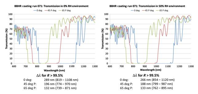
**Fig. 4** Measured transmission spectra of the BBHR coating of Run 071 for 0 deg AOI, and for 45-deg and 65-deg AOIs, PpoI, at 0% RH and 50% RH ambient conditions. The HR band,  $\Delta\lambda$ , for R > 99.5% is shown below the graphs for each measured spectrum.
