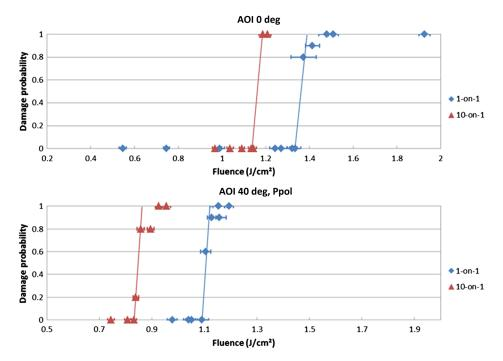
**Fig. 8** Damage probability versus fluence for 1-on-1 and 10-on-1 LIDT tests of the BBHR coating of Run 072, as measured by CEA-CESTA at 0-deg AOI and at 40-deg AOI, Ppol with 675 fs laser pulses of 1053-nm center wavelength. Solid lines are guides for the eyes. At 0-deg AOI, the 1-on-1 and 10-on-1 LIDTs are  $1.35\pm0.02$  and  $1.17\pm0.02$  J/cm², respectively. At 40-deg AOI, Ppol, the 1-on-1 and 10-on-1 LIDTs are  $1.10\pm0.01$  and  $0.83\pm0.01$  J/cm², respectively.
