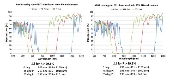
**Fig. 3** Measured transmission spectra of the BBHR coating of Run 072 for 0-deg AOI, and for 45-deg and 65-deg AOIs, PpoI, at 0% RH and 50% RH ambient conditions. The HR band,  $\Delta\lambda$ , for R > 99.5% is shown below the graphs for each measured spectrum.
