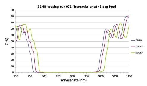
**Fig. 5** Measured transmission spectra of the BBHR coating of Run 071 at 45-deg AOI, Ppol, under 0%, 15%, and 50% RH conditions.
