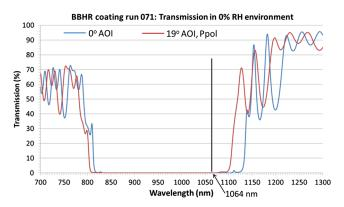
**Fig. 10** Measured transmission spectra of the BBHR coating of Run 071 at 0-deg AOI and at 19-deg AOI, PpoI under dry (0% RH) conditions. The thick black vertical line indicates 1064 nm, the center wavelength of the NIF-MEL 800 and 8 ps LIDT test laser pulses. It is between the central zone and edge of the HR band for 0-deg AOI, and near the HR band edge for 40-deg AOI, PpoI.
