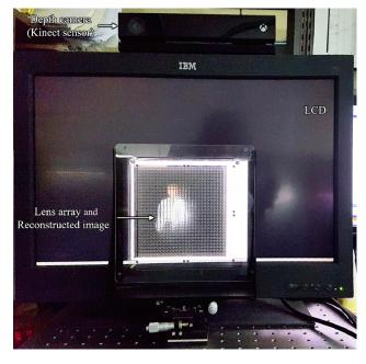
Fig. 11 The system implementation for the proposed method.
