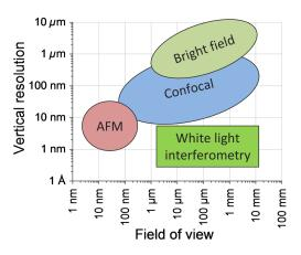
**Fig. 2** Comparison of imaging modalities used to collect 3-D topographical information from biofilms. Typically higher resolution necessarily limits the field of view. The axial resolution of interferometric imaging is independent of magnification, so high-resolution imaging is possible even with a large field of view. This is valuable for imaging biofilms, which are spatially heterogeneous.
