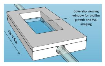
Fig. 3 3-D model of a flow cell used to grow and image biofilms. The viewing window serves as a support for biofilm growth and enables interferometric imaging. The viewing window is  $25 \times 50$  mm.
