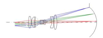
Fig. 6 The wide-angle eyepiece to broaden the field of view.
