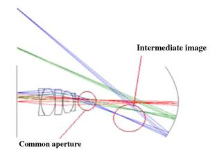
Fig. 7 The common aperture and intermediate image.
