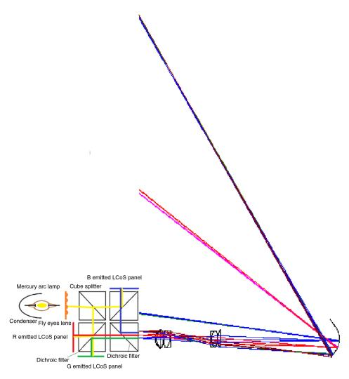
Fig. 11 The short throw ratio LCoS projection system with telecentric optics and Koehler illumination.
