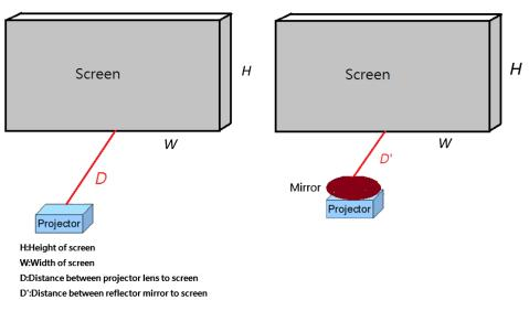
**Fig. 1** The definition of throw ratio (D/W) or (D'/W) for projectors.
