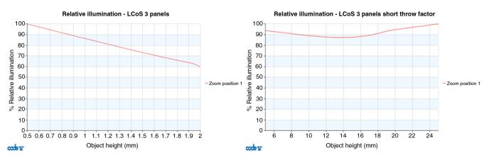
Fig. 14 The relative illumination before and after tuning the lens shape.
