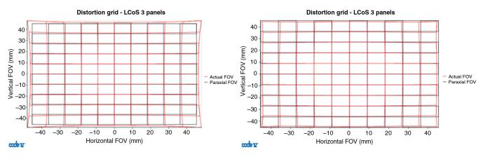
Fig. 15 The distortion before and after tuning the optical parameters.
