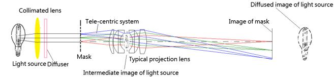
Fig. 2 Projection system with illumination and optics.
