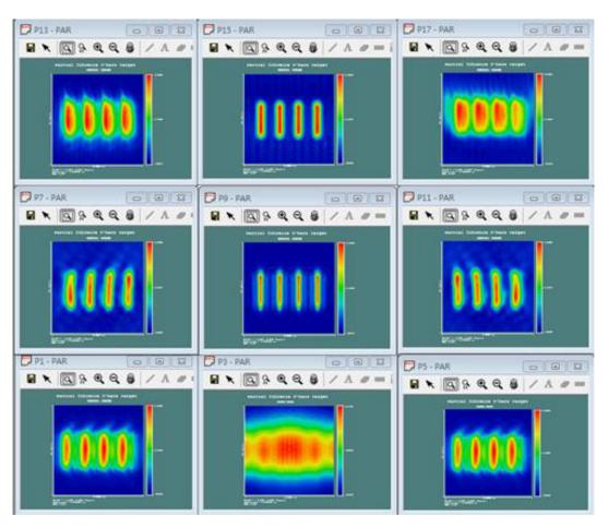
Fig. 18 Four-bar patterns with a pitch of 4  $\mu$ m projected in each field with respect to each field.
