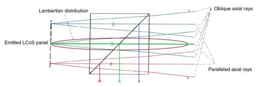
Fig. 5 The panel-emitted LCoS telecentric source.
