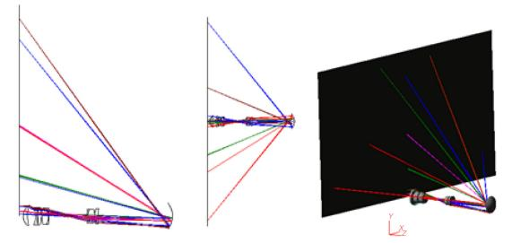
Fig. 12 The optical design for the short throw ratio projector.
