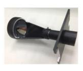
Fig. 19 Utmost Co. LCoS projection engine with self-designed optics and optomechatronic mount.
