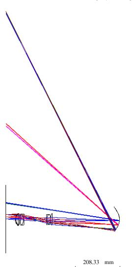
Fig. 8 The LCoS image is formed on the screen through the refractive lens and reflective mirror.
