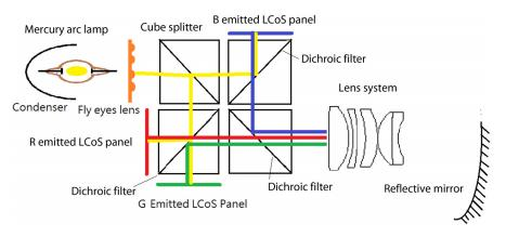
Fig. 3 Three-panel LCoS projection diagram.
