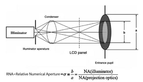
Fig. 9 The diagram of relative numerical aperture.
