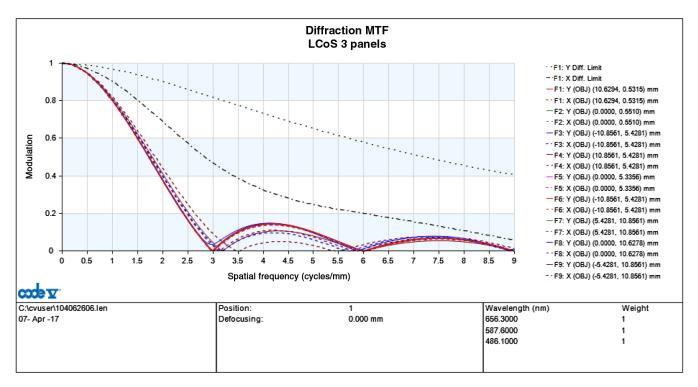
Fig. 17 The MTF of the short throw ratio projector.
