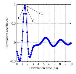
Fig. 4 Cross-correlation waveform between the reference and target signals.
