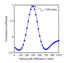
Fig. 8 Correlation waveform at the original target prism position.
