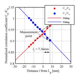
Fig. 11 Change of normalized correlation coefficient  $C_{\pm 1}/C_0$  after moving the target prism.
