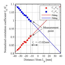
Fig. 9 Changes of normalized correlation coefficient  $C_{+1}/C_0$  at the original target prism position.
