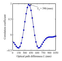
Fig. 10 Correlation waveform after moving the target prism.
