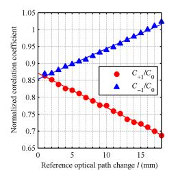
Fig. 7 Variation of normalized correlation coefficients at the ADC's sampling rate of 5 GS/s.
